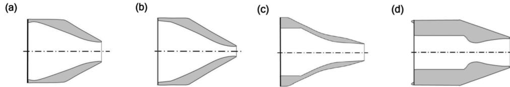
FIGURE 1. Schematic detailing the nozzle geometries investigated: (a) NASA Acoustic Reference Nozzle 1 (ARN1), (b) NASA Acoustic Reference Nozzle 2 (ARN2), (c) Small Metal Chevron (SMC000) nozzle, (d) Eggers Nozzle.
