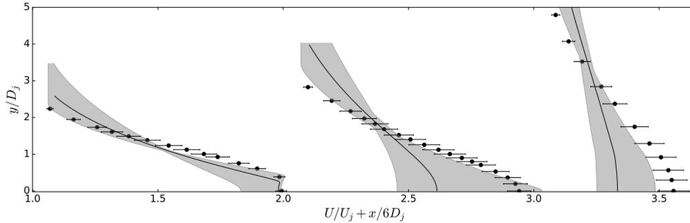
FIGURE 8. Mean axial velocity profiles in the nozzle jet exhaust for the Eggers experiment, delineated at  $x/D_j = 6, 12$  and  $24$ .
