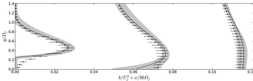
FIGURE 7. Turbulent kinetic energy profiles in the nozzle jet for Set point 23, delineated at  $x/D_j = 4, 8$  and  $12$ .
