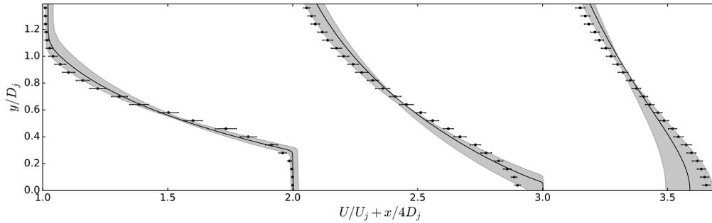
FIGURE 2. Mean axial velocity profiles in the nozzle jet exhaust for Set point 3. The dark lines represent the baseline predictions, the circles represent the PIV measurements of and the uncertainty bounds are shaded. The profiles are delineated at  $x/D_j = 4$ ,  $x/D_j = 8$ ,  $x/D_j = 12$ .
