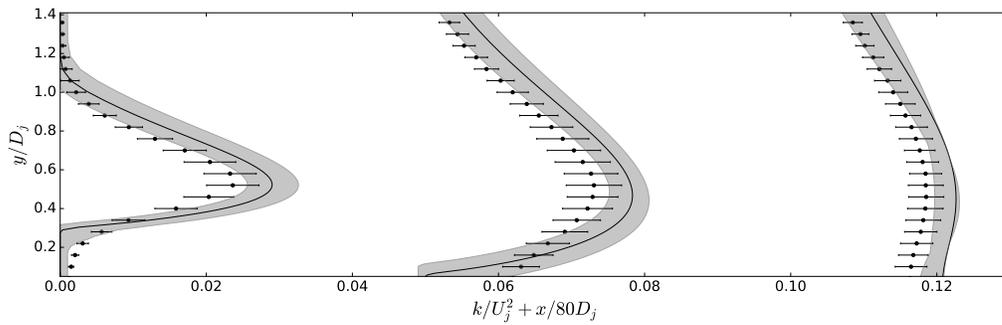
FIGURE 3. Turbulent kinetic energy profiles in the nozzle jet exhaust. The dark lines represent the baseline predictions, the circles represent the PIV measurements of and the uncertainty bounds are shaded. The profiles are delineated at  $x/D_j = 4$ ,  $x/D_j = 8$ ,  $x/D_j = 12$ .
