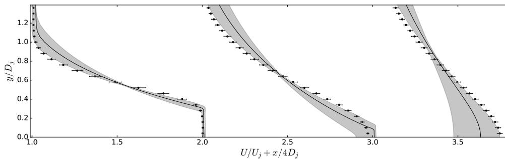
FIGURE 4. Mean axial velocity profiles in the nozzle jet for Setpoint 7, delineated at  $x/D_j = 4$ , 8 and 12.
