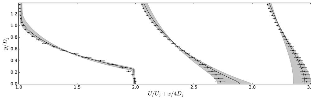
FIGURE 6. Mean axial velocity profiles in the nozzle jet for Set point 23, delineated at  $x/D_j = 4, 8$  and  $12$ .
