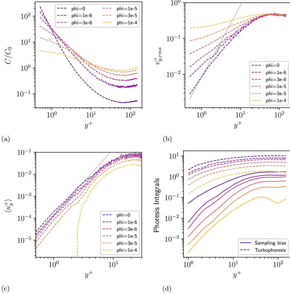
FIGURE 3. Statistics for  $St^+ = 32$  particles in a turbulent channel flow at  $Re_\tau = 150$  at various volume fractions. Descriptions of subfigures are the same as in Figure 1.
