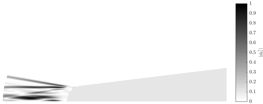
FIGURE 10. Magnitude of the streamwise mass flux component of the adjoint of the most unstable eigenfunction, |\hat{m}_1^\dagger| , for an azimuthal wavenumber of one. Note the cone is shaded light gray.
