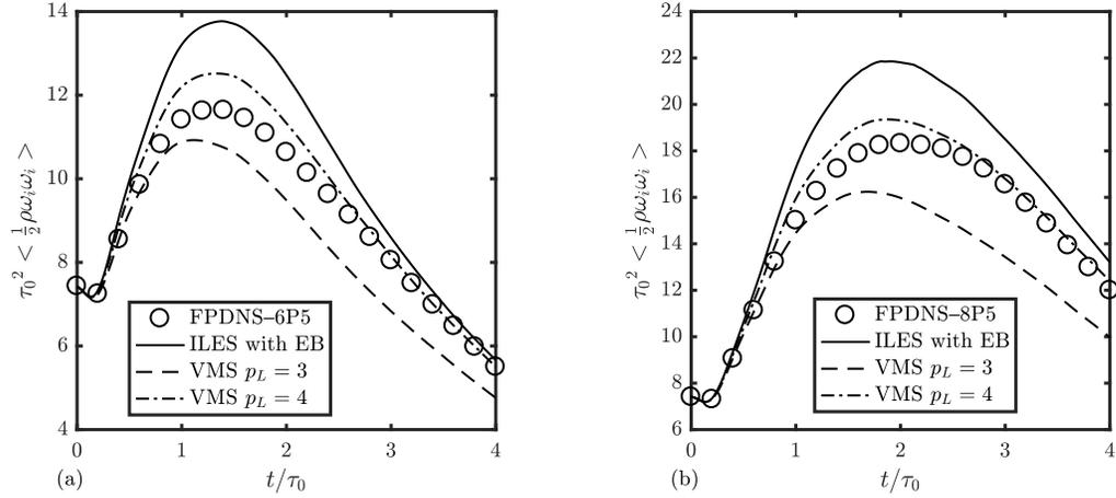
FIGURE 4. Comparison of enstrophy for LES and FPDNS: (a)  $Re_\lambda = 100$  with  $6^3$  elements and (b)  $Re_\lambda = 200$  with  $8^3$  elements.
