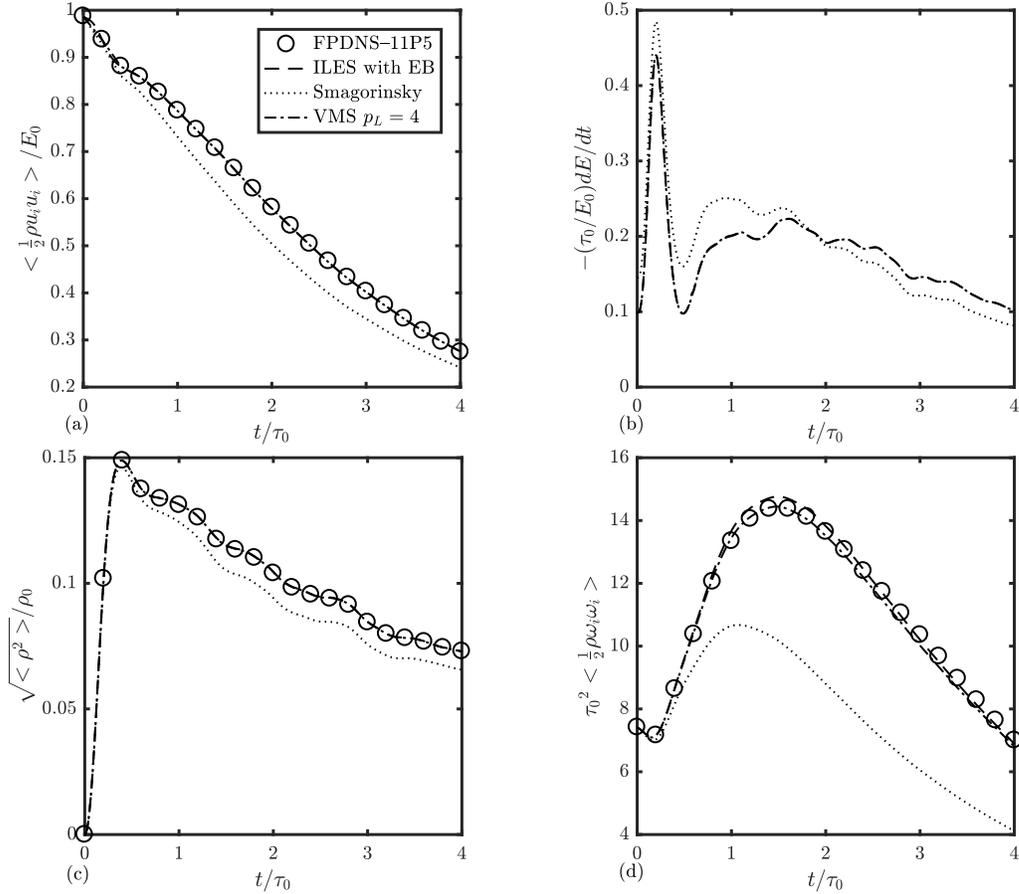
FIGURE 3. Comparison of LES (ILES and VMS including the standard Smagorinsky model) and FPDNS (reference LES) for  $11^3$  elements at  $Re_\lambda = 100$ : (a) turbulent kinetic energy, (b) decay rate, (c) density fluctuations, and (d) enstrophy.
