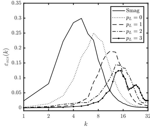
FIGURE 5. SGS dissipation spectrum at  $t/\tau = 1.6$  for  $11^3$  elements at  $Re_\lambda = 100$ .
