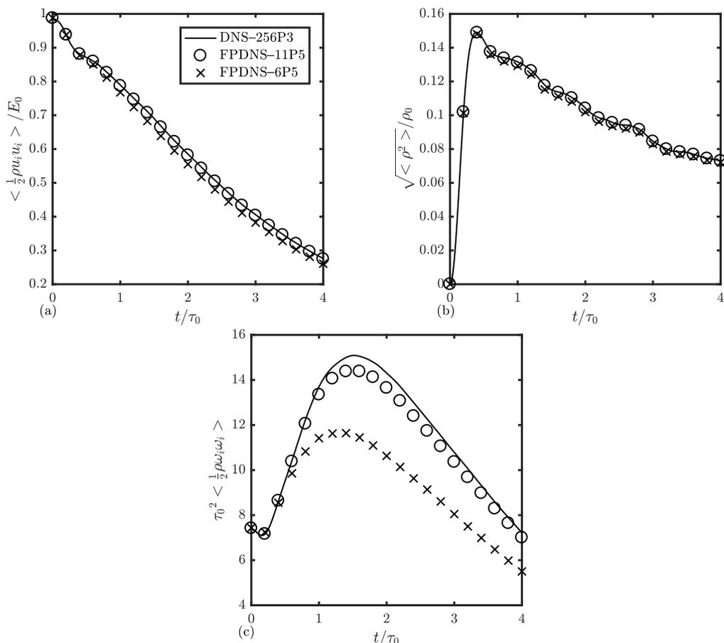
FIGURE 2. Comparison of DNS and FPDNS at  $Re_\lambda = 100$ : (a) turbulent kinetic energy, (b) density fluctuations, and (c) enstrophy.
