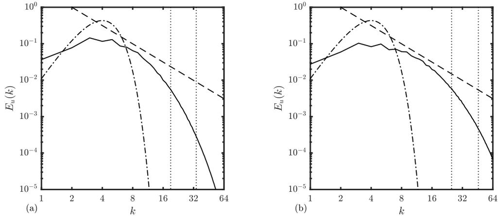
FIGURE 1. Velocity spectrum after four eddy turnover times with the LES resolution cutoff for (a)  $Re_\lambda = 100$  and (b)  $Re_\lambda = 200$ . Solid line: velocity spectrum; dashed line:  $-5/3$  slope; dotted lines: LES cutoffs; dash-dotted line: initial spectrum.
