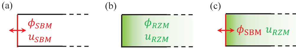
FIGURE 1. Wave generation methods (a) SBM, (b) RZM and (c) hybrid method. Color gradients represent the relaxation zone.
