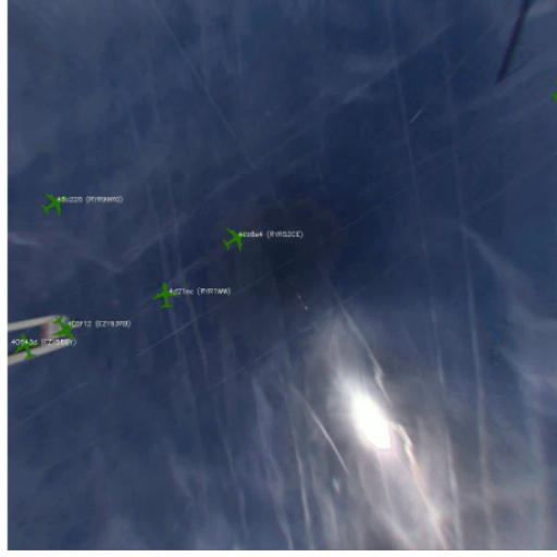
FIGURE 1. Ground-based camera image calibrated and overlapped with aircraft flight trajectories from ADS-B data.
