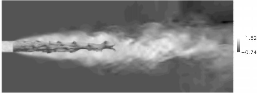
FIGURE 5. Instantaneous flame front location and axial velocity.
