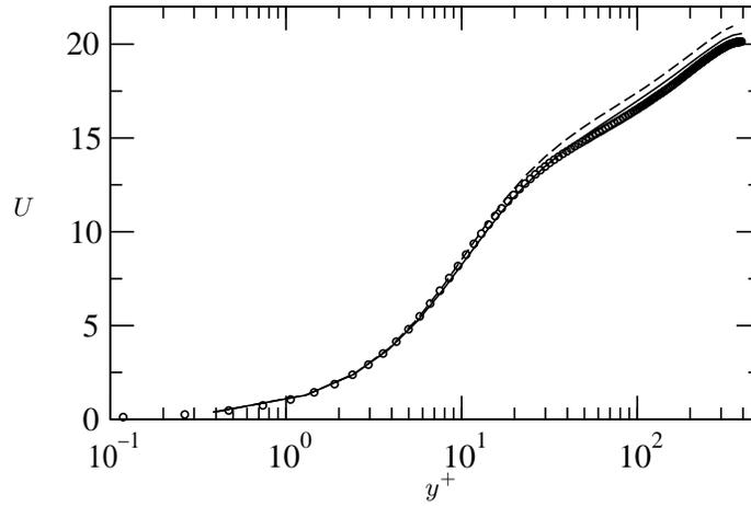
FIGURE 4. Mean velocity profile  $U$  as a function of the distance to the wall  $y^+$ .  $Re_\tau=395$ .  $\circ$ : DNS spectral code,  $\text{—}$ : LES 4th order FD code and  $\text{---}$ : LES 2nd order FD code.
