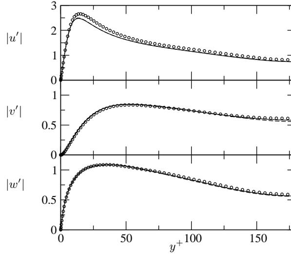
FIGURE 2. Velocity fluctuations in streamwise  $|u'|$ , wall normal  $|v'|$  and spanwise  $|w'|$  direction as a function of the distance to the wall  $y^+$ .  $Re_\tau=180$ . DNS  $\circ$ : spectral code, — : 4th order FD code and - - - : 2nd order FD code.
