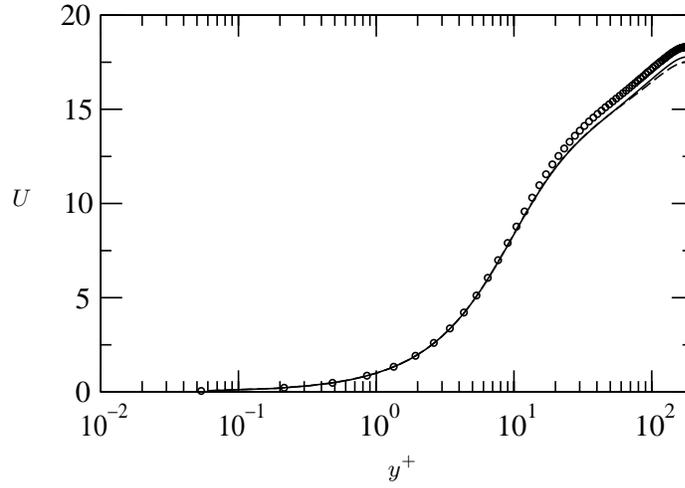
FIGURE 1. Mean velocity profile  $U$  as a function of the distance to the wall  $y^+$ .  $Re_\tau=180$ . DNS  $\circ$ : spectral code, — : 4th order FD code and - - - : 2nd order FD code.
