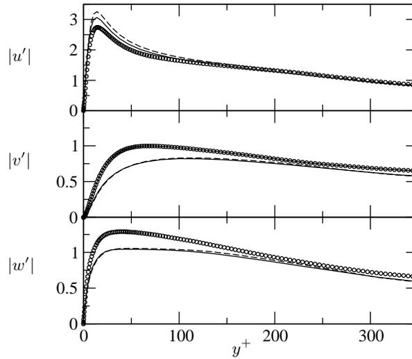
FIGURE 5. Velocity fluctuations in streamwise  $-\overline{u'^2}$ , wall normal  $|v'|$  and spanwise direction  $|w'|$  as a function of the distance to the wall  $y^+$ .  $Re_\tau=395$ .  $\circ$ : DNS spectral code,  $\text{—}$ : LES 4th order FD code and  $\text{---}$ : LES 2nd order FD code.
