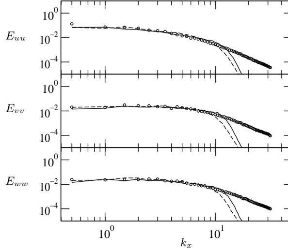
FIGURE 3. Energy spectrum of the streamwise  $E_{uu}$ , wall normal  $E_{vv}$  and spanwise  $E_{ww}$  velocity correlation as a function of the streamwise wavenumber  $k_x$ .  $Re_\tau=180$  at  $y^+ \approx 180$ . DNS  $\circ$ : spectral code, — : 4th order FD code and - - - : 2nd order FD code.
