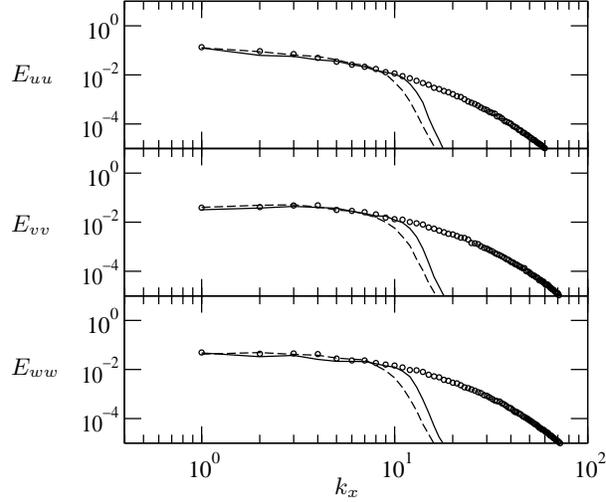
FIGURE 6. Energy spectrum of the streamwise  $E_{uu}$ , wall normal  $E_{vv}$  and spanwise  $E_{ww}$  velocity correlation as a function of the streamwise wavenumber  $k_x$ .  $Re_{\tau}=395$  at  $y^+ \approx 395$ .  $\circ$ : DNS spectral code,  $\text{—}$ : LES 4th order FD code and  $\text{- - -}$ : LES 2nd order FD code.
