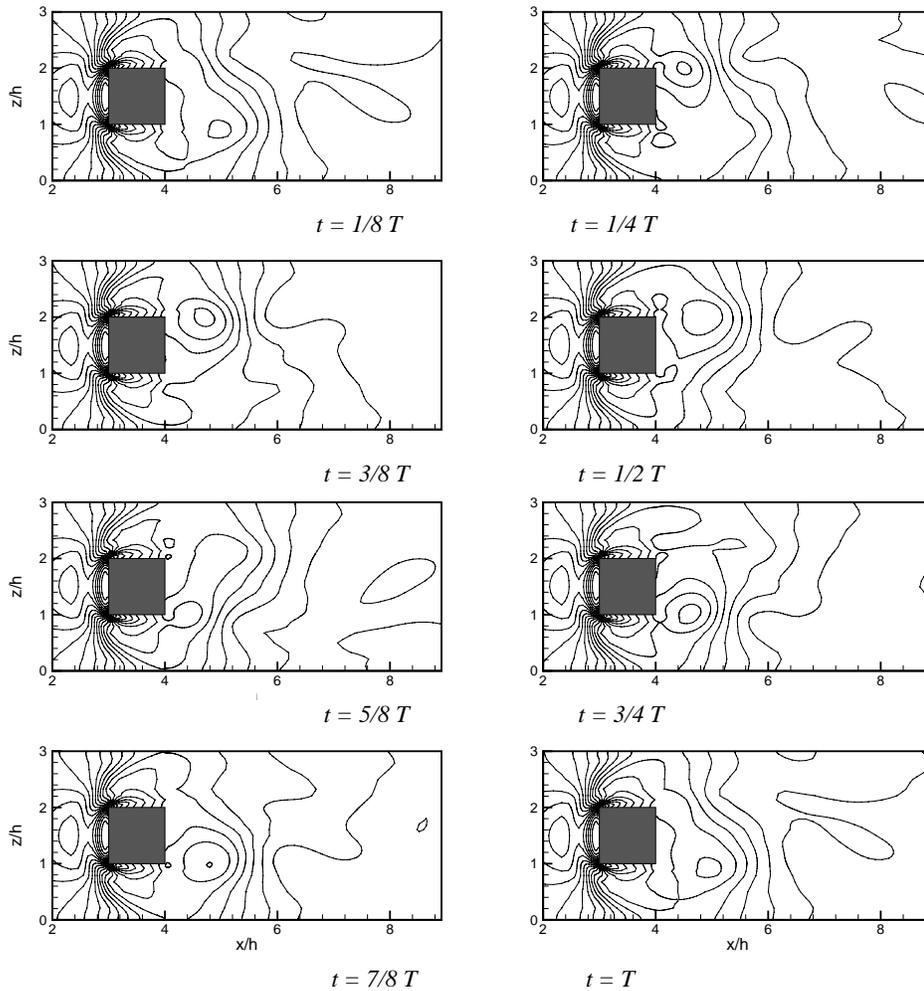
FIGURE 5. Time-history of the pressure distribution on the floor.
