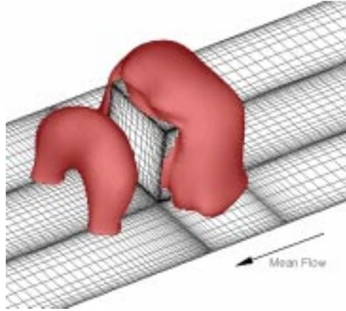
FIGURE 4. Visualization of the arch-vortex in the wake using an isobar surface.
