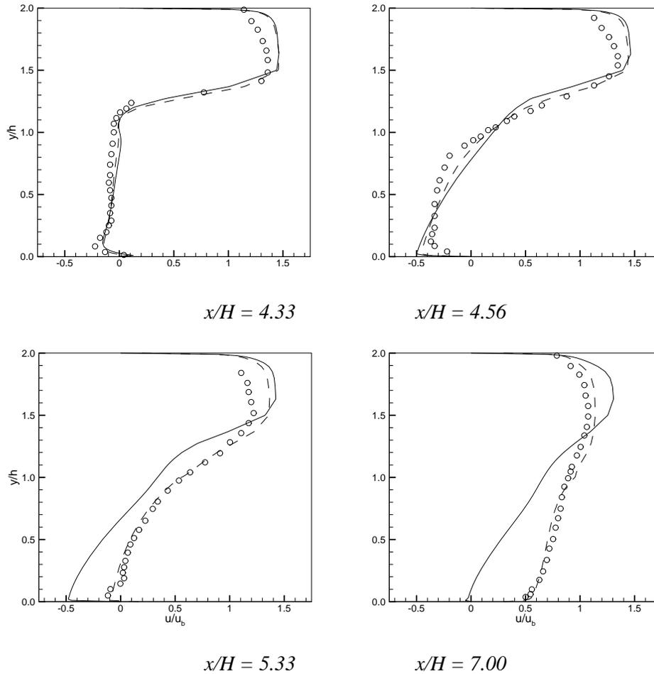
FIGURE 6. Streamwise velocity profiles in the symmetry plane. Symbols: — : steady solution; ---- : unsteady solution; o : experiments.
