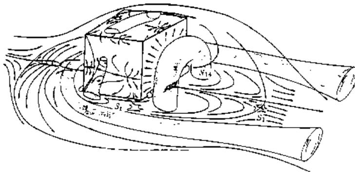
FIGURE 1. Schematic representation of the main flow features (Hussein & Martinuzzi, 1996).
