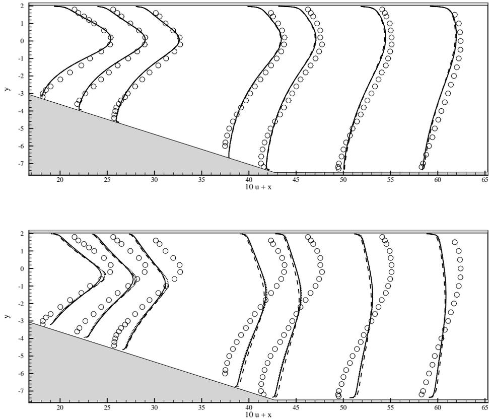
FIGURE 4. Streamwise velocity profiles. Top:  $\overline{v^2} - f$  model; bottom: Low-Reynolds  $k-\epsilon$  model - Symbols:  $\circ$  Experiments, — CFX, - - - - Fluent, ····· Star-CD
