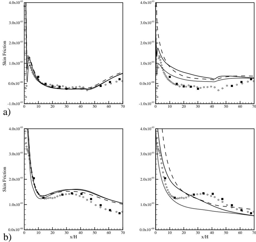
FIGURE 6. Skin friction distribution. Left column:  $\overline{v^2} - f$  model; right column: Low-Reynolds  $k-\epsilon$  model. a) Lower wall; b) Upper wall - Symbols:  $\circ$  LES,  $\blacksquare$  Experiments,  $\text{—}$  CFX,  $\text{- - -}$  Fluent,  $\cdots$  Star-CD
