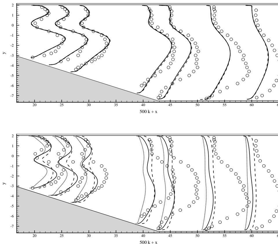
FIGURE 5. Turbulent kinetic energy profiles. Top:  $\overline{v^2} - f$  model; bottom: Low-Reynolds  $k-\epsilon$  model - Symbols:  $\circ$  Experiments, — CFX, ---- Fluent, ..... Star-CD
