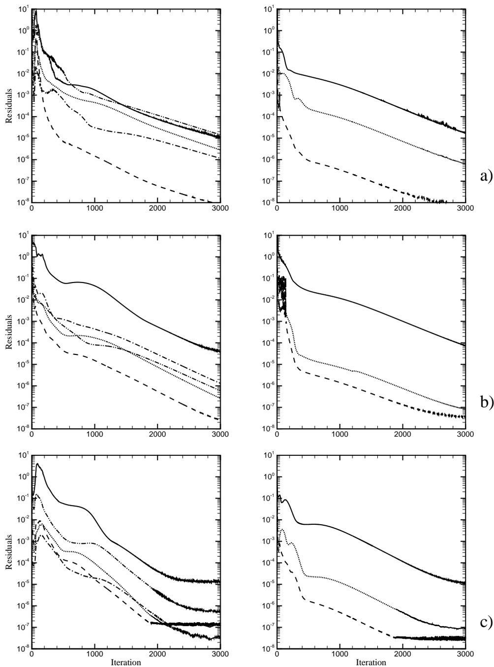
FIGURE 3. Convergence history ( $L_\infty$  Norm). Left column:  $\overline{v^2} - f$  model; right column: Low-Reynolds  $k-\epsilon$  model. a) CFX v4.3; b) Fluent v5.3; c) Star-CD v3.1. - Symbols: — x-momentum, .....  $k$ , - - -  $\epsilon$ , - · -  $v^2$ , - - -  $f$
