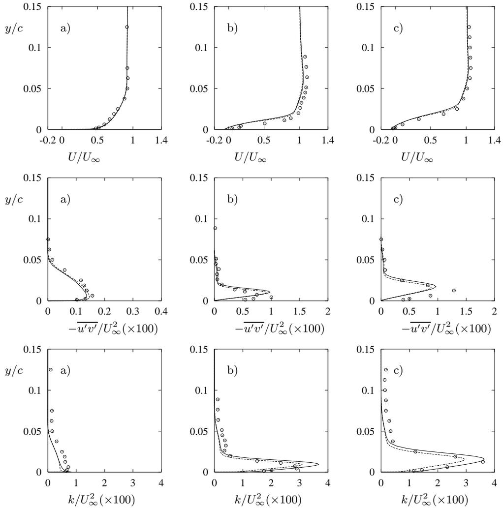
FIGURE 2. Bachalo-Johnson bump: velocity, shear-stress and turbulent kinetic energy;  $v^2$ - $f$ :
