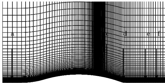
FIGURE 3. Bachalo-Johnson bump: computational mesh.  $x/c = -0.250$  (a),  $0.750$  (b),  $0.813$  (c),
