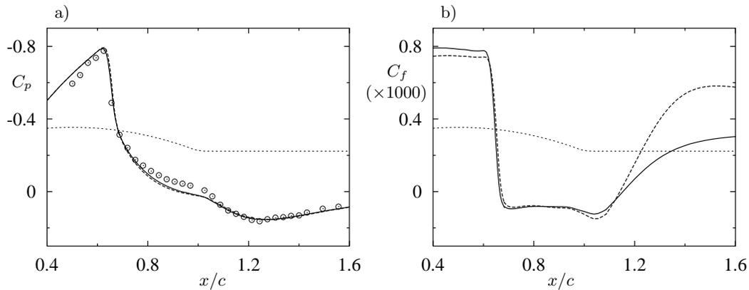
FIGURE 5. Bachalo-Johnson bump: a) pressure and b) skin friction dist.;  $v^2$ - $f$ : — : version A, - - - : version B,  $\circ$  : expt.
