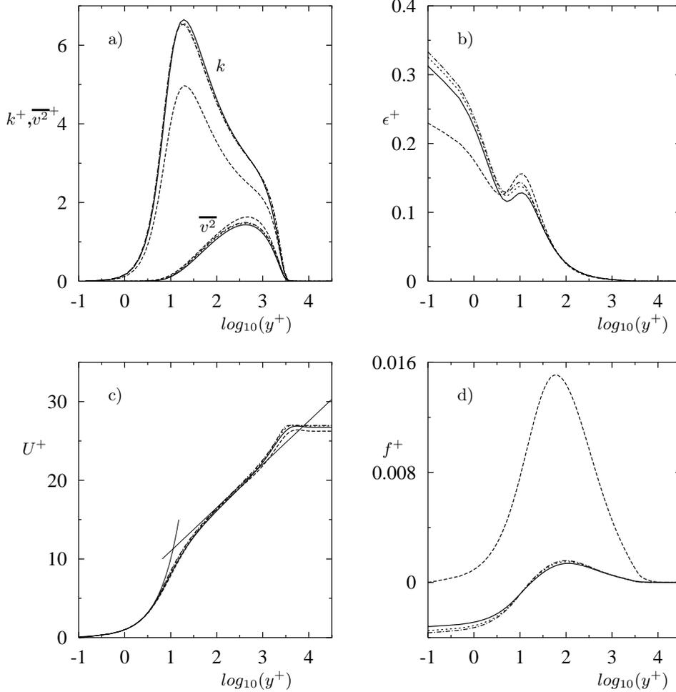
FIGURE 1. Profiles of a)  $k$  and  $\overline{v^2}$  b)  $\epsilon$ , c)  $U^+$  and d)  $f$  for flow over a flat plate;  $v^2$ - $f$ : --- : version A, CFL3D; ..... : version A, TFLO, VIS4=0.3; — : version A, TFLO, VIS4=1.0 -.-.- : version B, TFLO, VIS4=1.0).
