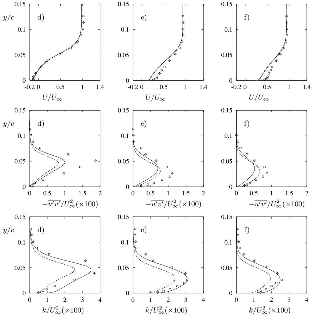
FIGURE 4. Bachalo-Johnson bump: velocity, shear-stress, and turbulent kinetic energy; (continuation);  $v^2$ - $f$ : — : version A, - - - : version B,  $\circ$  : expt.
