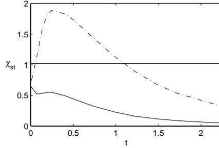
FIGURE 1. The time evolution of  $\chi_{st}$ . Here  $\chi_{st}$  is the scalar dissipation rate at  $Z = Z_{st} = 0.5$ .  $\text{—}$  :  $\langle \chi_{st} \rangle$ ,  $\text{- - -}$  : 99% envelope of the fluctuations of  $\chi_{st}$ . The horizontal line is drawn at  $\chi_{st} = \chi_q = 1.02$ . This is the largest possible value of  $\chi_{st}$  where the steady flamelet equation has a burning solution. The numerical value refers to the chemistry parameters shown in Table 2.
