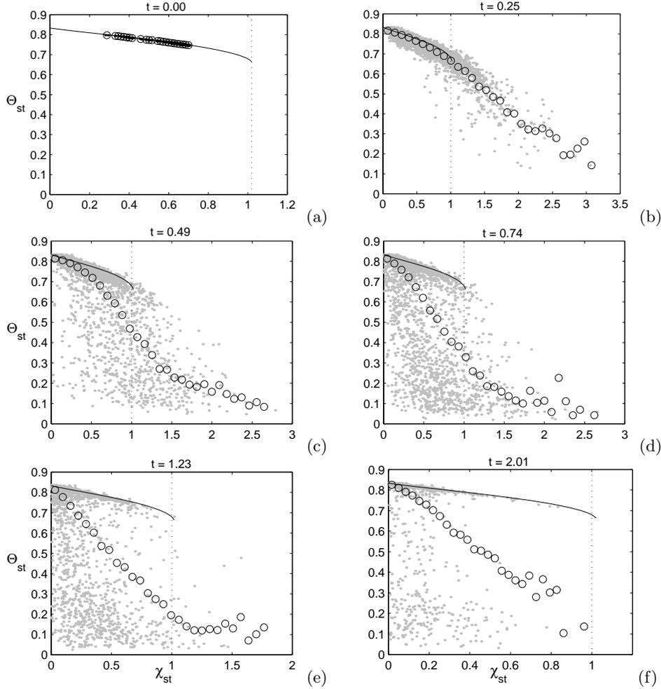
FIGURE 3. Extinction-reignition behavior on the  $Z_{st}$  surface. — : burning solution of the steady-flamelet equation.  $\circ$  : average temperature for chosen values of the scalar dissipation rate ( $\langle \Theta | Z_{st}, \chi_{st} \rangle$ ). The grey dots represent the temperature of 5000 randomly selected flame elements. The vertical dotted line is at  $\chi_{st} = \chi_q$ .
