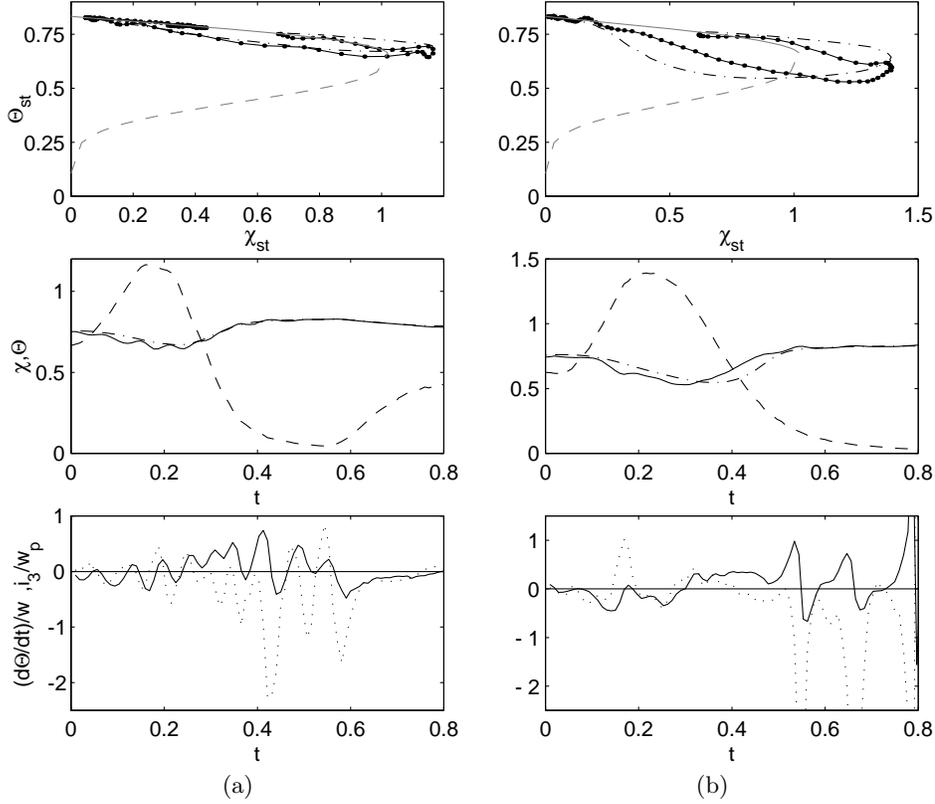
FIGURE 5. Various flame element histories with different patterns of extinction-reignition. Top two figures: — : temperature data; —·— : TFL model results; grey — and — — : burning and unstable branches of the SFL solution; — — — : scalar dissipation rate. Bottom figure: — :  $(d\Theta/dt)/w$  from DNS data; ····· :  $i_3/w$  term.
