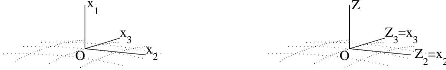
FIGURE 2. The local coordinate system used in flamelet modeling. Point O is fixed on the stoichiometric surface.
