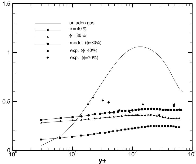
FIGURE 3. Particle wall-normal fluctuations: mean-square intensity profiles, in wall units
