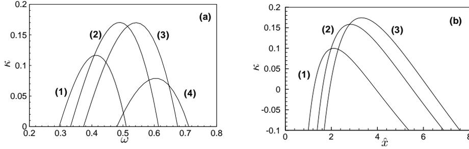
FIGURE 3. Inviscid growth rates  $\kappa$  of localized modes for  $B_0 = -6$ . (a)  $\kappa$  v.s.  $\omega$  at  $\hat{x} = 2, 3, 4$  and  $6$ , represented by curves (1)-(4) respectively. (b)  $\kappa$  v.s.  $\hat{x}$  for  $\omega = 0.37, 0.45$  and  $0.50$  represented by curves (1)-(3) respectively.
