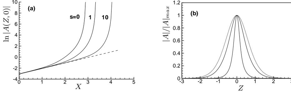
FIGURE 5. Nonlinear evolution of a localized mode ( $\omega = 0.8$ ,  $\hat{x} = 6.5$ ). (a) The amplitude on the symmetry plane  $\ln |A(X, 0)|$  v.s.  $X$  for  $s = 0$  (purely inviscid case), 1 and 10.  $\cdots$  the linear limit. (b) Spanwise distribution of  $|A|$  at  $X = 3.02, 3.54$  for  $s = 1$ , showing self-focusing as  $X$  increases. The least ‘compact’ of the three curves corresponds to the linear limit.
