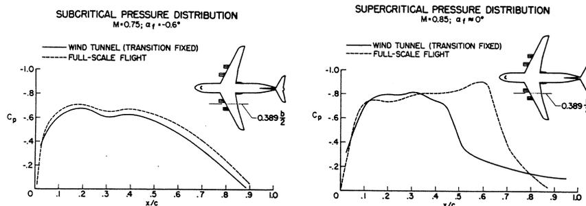
FIGURE 3. Comparison of C-141 wing pressure distributions between wind tunnel and flight for, (a) subcritical and (b) supercritical flow (Elsenaar (1988b))
