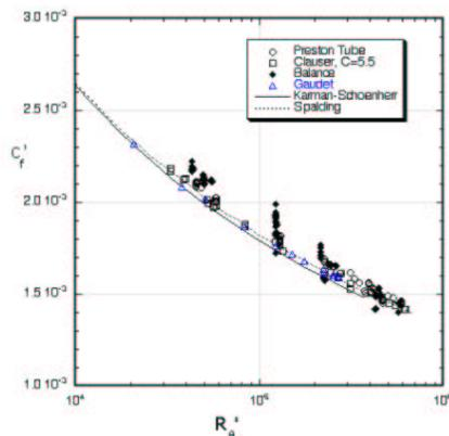
FIGURE 7. Comparison of three measurement techniques of skin friction with the data of Gaudet (1984) and with the predictions of Kármán-Schoenherr and Spalding (Watson *et al.* (2000))
