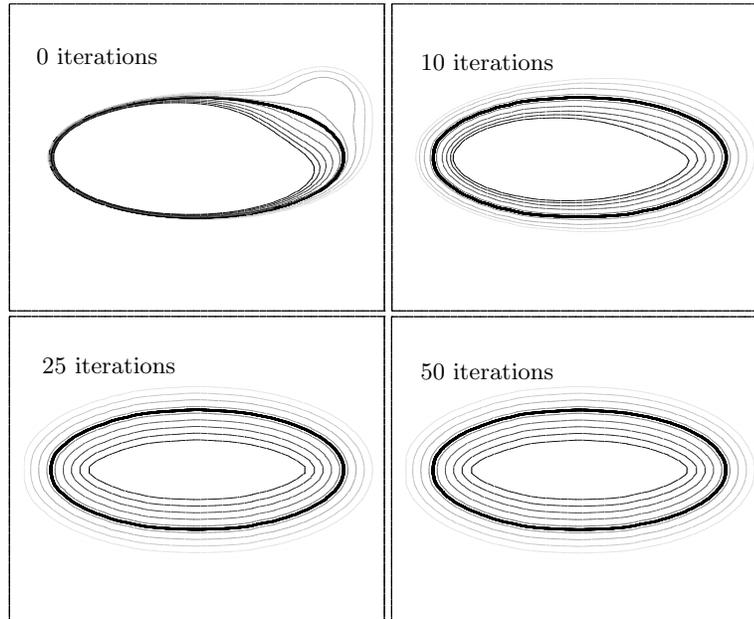
FIGURE 2. One time reinitialization with sign function defined by (3.10) on a  $50 \times 50$  grid. From left to right and top to bottom, reinitialized field after 0, 10, 25 and 50 iterations. The  $G_0 = 0$  level is displayed as a bold line.
