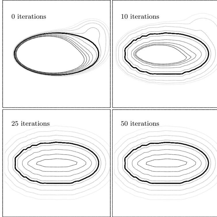
FIGURE 1. One time reinitialization with sign function defined by (3.3) on a  $50 \times 50$  grid. From left to right and top to bottom, reinitialized field after 0, 10, 25 and 50 iterations. The  $G_0 = 0$  level is displayed as a bold line.
