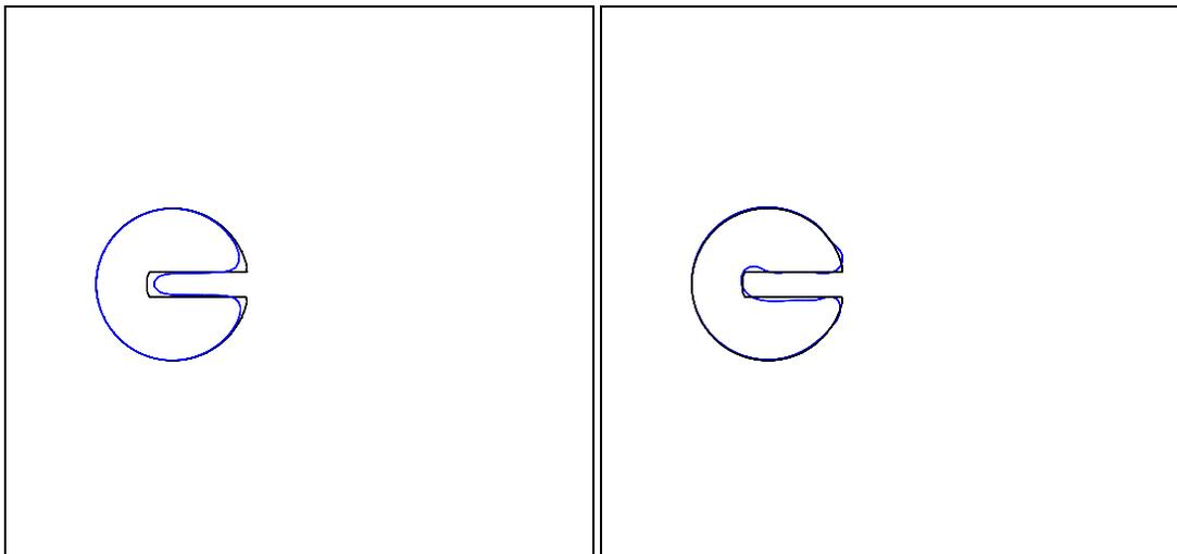
FIGURE 3. Zalesak's problem after one full revolution on a  $100 \times 100$  grid, reinitialization alone (left) and reinitialization with volume-preservation constraint (right).
