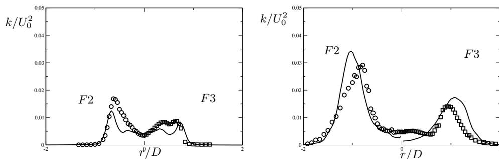
FIGURE 5. Reacting flow. Radial profiles of turbulent kinetic energy. Solid lines denote the LES results, symbols denote experimental data. Stations:  $x/D = 2.5$  (left) and  $x/D = 6.5$  (right).
