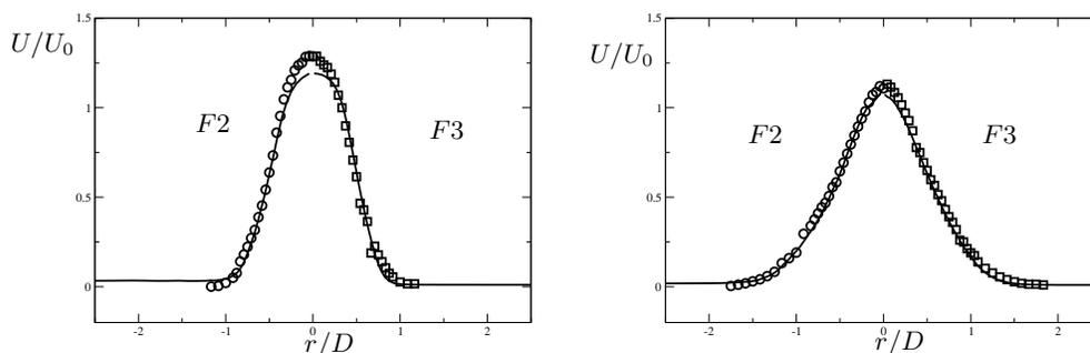
FIGURE 2. Cold flow. Radial profiles of mean axial velocity. Solid lines denote the LES results, symbols denote experimental data. Stations:  $x/D = 2.5$  (left) and  $x/D = 6.5$  (right).
