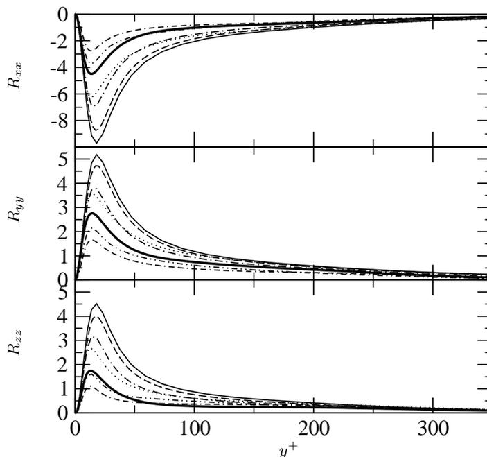
FIGURE 5. Reduced (deviatoric) turbulence intensities in streamwise  $R_{xx}$ , wall-normal  $R_{yy}$ , and spanwise  $R_{zz}$  directions. — : DNS, — : DSM (64,49,48), - - - : DSM (128,97,96), - · - : DMM (64,49,48), ····· : DMM (128,97,96), - · - · : DRM (64,49,48), and · - · - : DRM (128,97,96).
