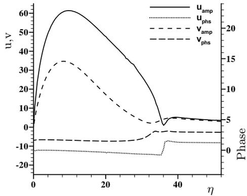
FIGURE 4.  $u$  and  $v$  eigensolutions at  $R_x=1000$  for two-dimensional disturbances at  $F=3.6416 \cdot 10^{-5}$ .  $u_{amp}$  ( — ),  $v_{amp}$  ( - - - ),  $u_{phs}$  ( ..... ),  $v_{phs}$  ( - · - · )
