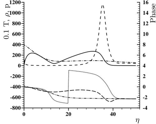
FIGURE 5.  $t$ ,  $\rho$  and  $p$  eigensolutions at  $R_x=1000$  for two-dimensional disturbances at  $F=3.6416 \cdot 10^{-5}$ .  $t$  is scaled by a factor of 0.1.  $t_{amp}$  ( — ),  $\rho_{amp}$  ( - - - ),  $p_{amp}$  ( - · - · ),  $t_{phs}$  ( ..... ),  $\rho_{phs}$  ( - · - · - · ),  $p_{phs}$  ( - - - - )
