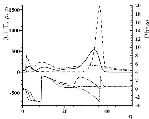
FIGURE 7.  $t$ ,  $\rho$  and  $p$  eigensolutions at  $R_x=2450$  for two-dimensional disturbances at  $F=3.6416 \cdot 10^{-5}$ .  $t$  is scaled by a factor of 0.1.  $t_{amp}$  ( — ),  $\rho_{amp}$  ( - - - ),  $p_{amp}$  ( - · - · ),  $t_{phs}$  ( ····· ),  $\rho_{phs}$  ( - · - · ),  $p_{phs}$  ( - - - - ).
