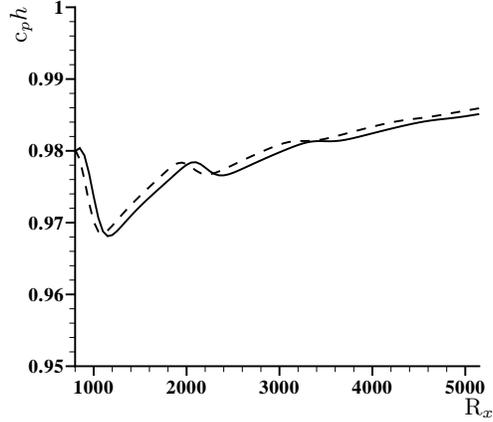
FIGURE 3. phase velocity  $c_p h$  vs. the downstream direction for two-dimensional disturbances at  $F=3.6416 \cdot 10^{-5}$  ( — ) and  $F=3.9 \cdot 10^{-5}$  ( - - - )
