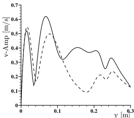
FIGURE 10. Comparison of simulation (—) and Linear Stability results (----) of the wall-normal velocity  $v$  at  $R_x = 2800$
