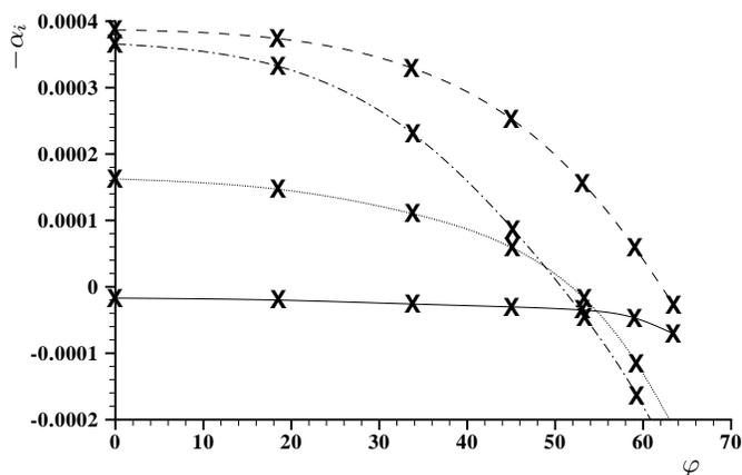
FIGURE 8. spatial amplification rate  $-\alpha_i$  vs. wave propagation angle  $\varphi$  for  $F=3.6416 \cdot 10^{-5}$ .
