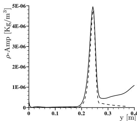
FIGURE 12. Comparison of simulation (—) and Linear Stability results (----) of the density  $\rho$  at  $R_x = 2800$
