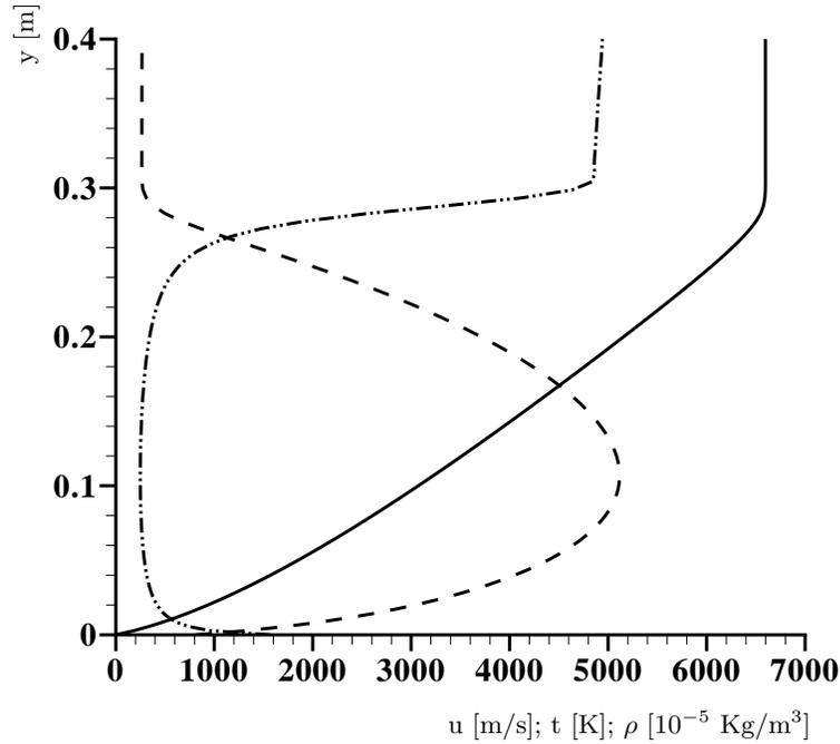
FIGURE 1. Wall-normal profiles of streamwise-velocity, temperature and density for  $Re_x=4 \cdot 10^6$  in dimensional units. Note that the density has been multiplied by a factor of  $10^5$  to show on the graph.
