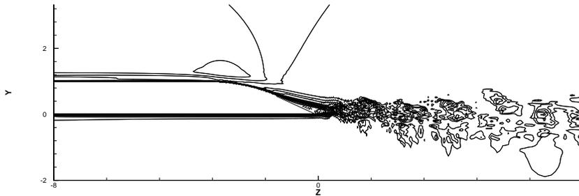
FIGURE 3. Flow past a hydrofoil trailing edge. The contours ( $-0.2$  to  $1.2$  with increment  $0.08$ ) represent the instantaneous streamwise velocity.
