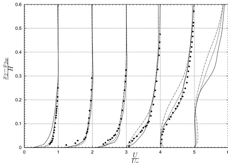
FIGURE 4. Mean velocity magnitude at (from left to right)  $x_1/H = -3.125, -2.125, -1.625, -0.625, 0$ .  $\bullet$ , experiment (Blake 1975); ----, full LES (Wang & Moin 2000); —, present calculation; — · —, LES with wall model (Wang & Moin 2002).
