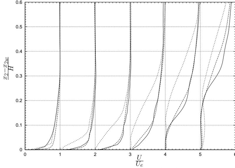
FIGURE 5. Mean velocity magnitude at (from left to right)  $x_1/H = -3.125, -2.125, -1.625, -0.625, 0, 0.625$ . ----, full LES (Wang & Moin 2000); —, present LES with wall model; - - -, present LES without wall model.
