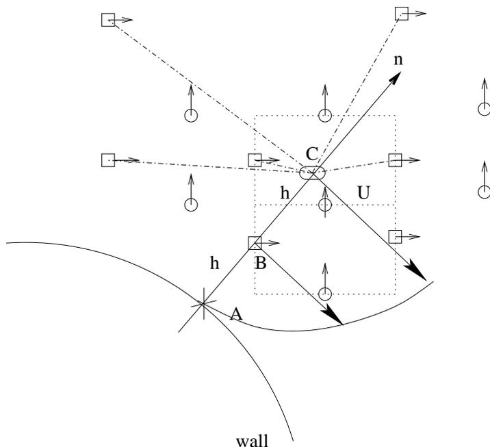
FIGURE 1. Interpolation procedure:  $\square$ , streamwise velocity node;  $\circ$ , vertical velocity node.  $n$  is normal to the wall from first external point B.  $U$  is the tangential velocity interpolated at point C, used as boundary condition for the wall model.
