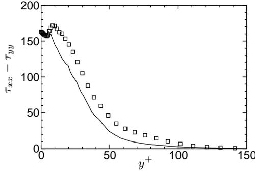
FIGURE 1. *Left*: Normal stress profiles of the viscoelastic simulation L100W120MC,  $\square$ , compared to the Brownian dynamic simulation,  $\text{—}$ .
