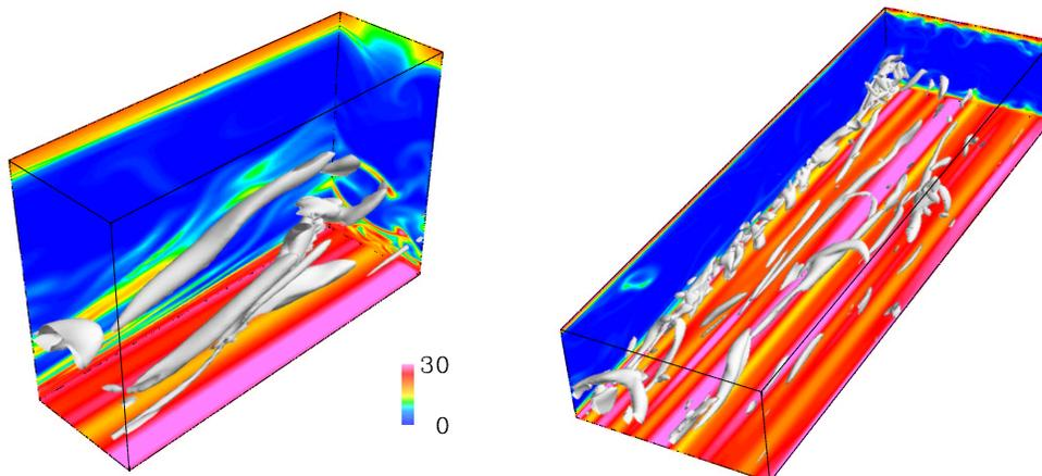
FIGURE 4. Snapshot of vortices identified by the  $Q$ -criterion (Dubief & Delcayre 2000) and the trace ( $c_{kk}/L^2 \times 100$ ). *Left* L60W84MC; *right* L60W84LC. Vortices are only shown in the lower half of the domain.
