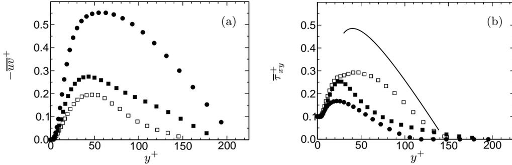
FIGURE 3. Reynolds shear stress (3a) and polymer stress (3b) normalized by  $u_\tau$  and  $\nu$ . Symbols are defined in Table 1. In Fig. 3b, — represents the contribution the polymer stress would have to Eq. (3.1) in the case of MDR defined by the velocity profile  $U^+ = 11.7 \ln(y^+) - 17$  and  $-\overline{uv}^+ = 0$ .
