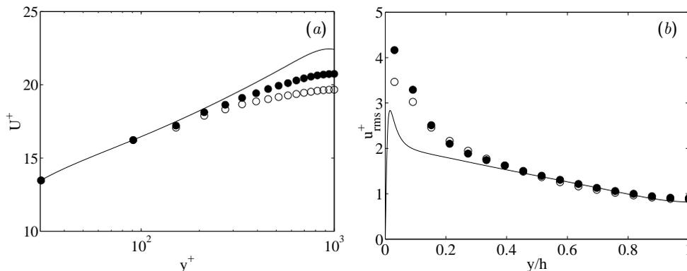
FIGURE 2. Profiles of (a) the mean velocities and (b) the streamwise velocity fluctuations for a smooth-walled channel at  $Re_\tau \approx 1000$ , using different cost functions.  $\circ$ , case **S1**;  $\bullet$ , case **S2**; —, direct simulation (del Álamo *et al.* 2003).
