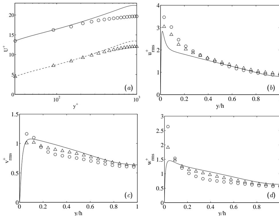
FIGURE 3. (a) Mean velocity profiles. (b) Streamwise velocity fluctuations. (c) Wall-normal velocity fluctuations. (d) Spanwise velocity fluctuations. —, smooth wall DNS,  $Re_\tau = 950$ ; ---, reference velocity profile for the rough case;  $\circ$ , case **S1**;  $\triangle$ , case **R1**.
