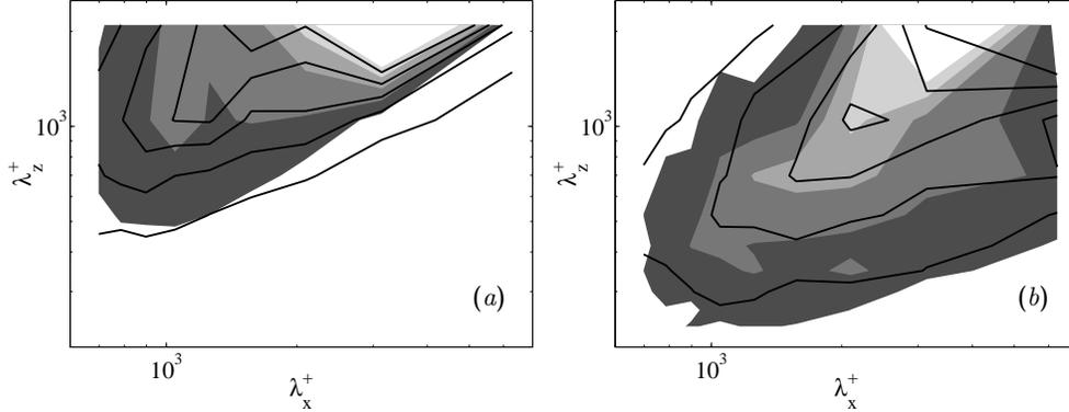
FIGURE 6. Two-dimensional premultiplied spectra of the stresses at the wall as functions of the streamwise and spanwise wavelengths. (a)  $E_{xy}$ , (b)  $E_{zy}$ . Shaded contours are from the **S1** case and lines are from **R1**. Each spectrum is normalized with its maximum.
