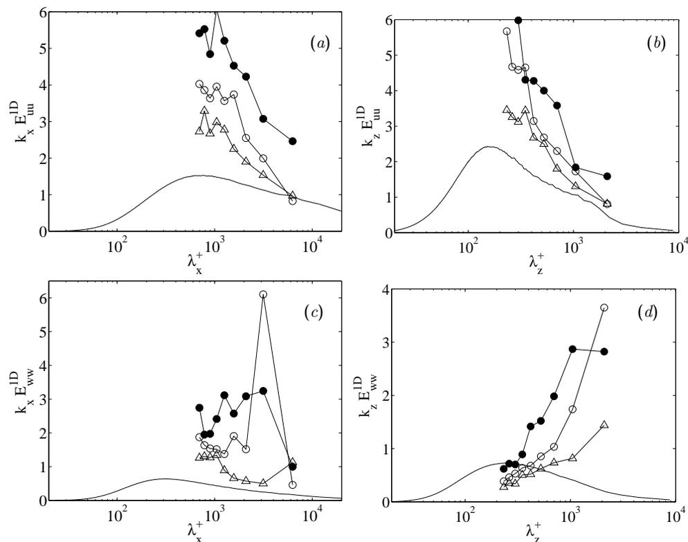
FIGURE 7. One-dimensional premultiplied velocities spectra at  $y^+ = 30$ , normalized in wall units and plotted as functions of the wavelengths  $\lambda_x$  (a, c) and  $\lambda_z$  (b, d). (a) and (b), streamwise component; (c) and (d) spanwise component. —, DNS;  $\circ$ , case S1;  $\bullet$ , case S2;  $\triangle$ , case R1.
