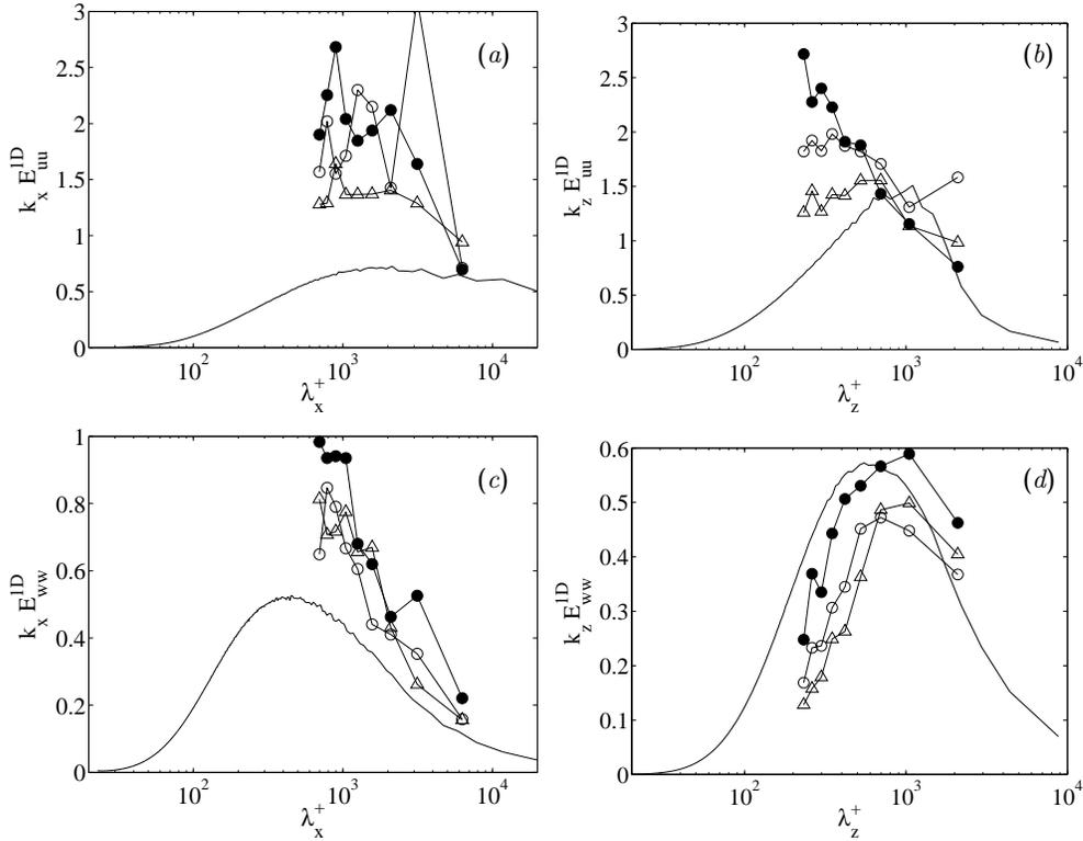
FIGURE 8. One-dimensional premultiplied velocities spectra at  $y^+ = 150$ , normalized in wall units and plotted as functions of the wavelengths  $\lambda_x$  (a, c) and  $\lambda_z$  (b, d). (a) and (b), streamwise component; (c) and (d) spanwise component. —, DNS;  $\circ$ , case S1;  $\bullet$ , case S2;  $\triangle$ , case R1.
