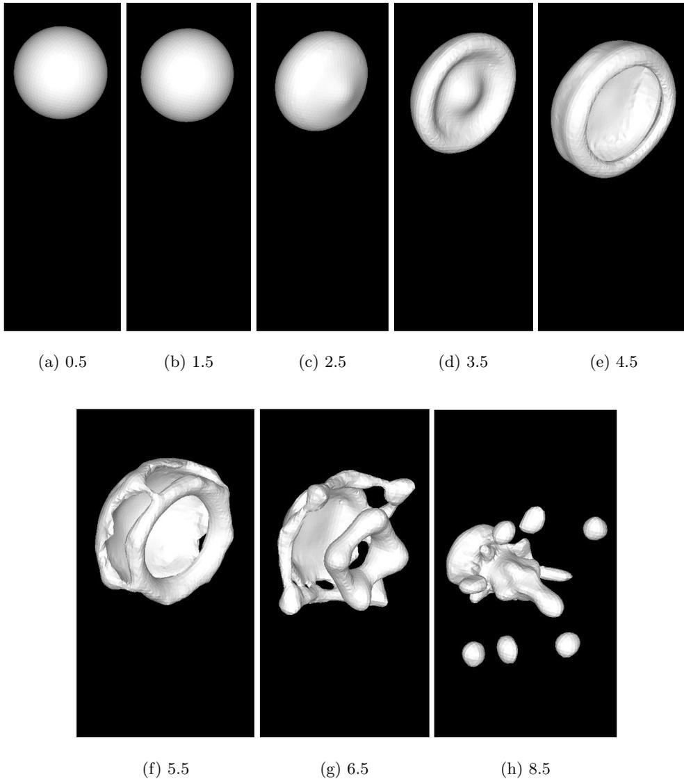
FIGURE 4. Breakup of an initially spherical drop in an impulsively accelerated field. The number below each figure indicates the non-dimensional time  $tU/D$ . Free stream velocity is from top-left-back to lower-right-front. Properties for this simulation are as follows:  $Re = \rho_g DU/\mu_g = 1000$ ,  $We = \rho_g U^2 D/\sigma = 20$ ,  $Oh = \mu_l/\sqrt{\rho_l \sigma D} = 0.007$ .
