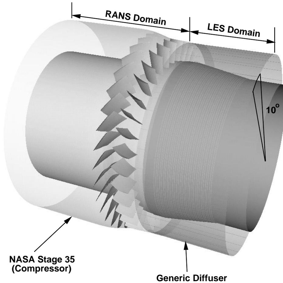
FIGURE 4. Geometry of the coupled NASA stage 35/prediffuser geometry. RANS domain includes one stage of a compressor, consisting of one rotor and one stator. LES domain includes the diffuser. A  $10^\circ$  axi-symmetric sector is computed.
