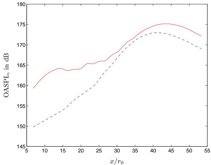
FIGURE 7. Overall sound pressure levels recorded along a cylindrical surface at a distance of  $6D_j$  from the jet centerline. Pressure matched jet with  $M_j = 1.95$ ,  $- -$ ; imperfectly expanded jet  $-$ .
