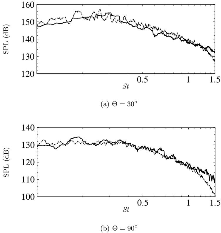
FIGURE 4. Narrowband spectra at  $\mathcal{R} = 30D_j$  for the Mach 2.0 unheated jet M15TR056. Lighthill (total), —; Kirchhoff Surface, - · - ·.
