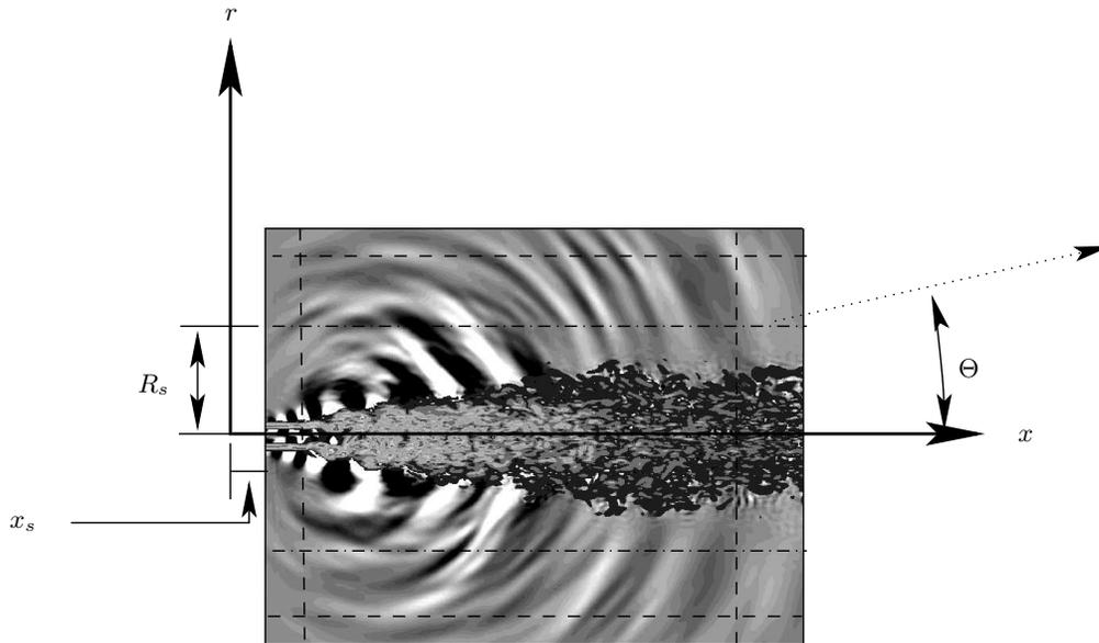
FIGURE 1. Schematic of calculation domain showing major features. The central region contains the LES domain and the sponge (---) and Kirchhoff surface surfaces (- · -).
