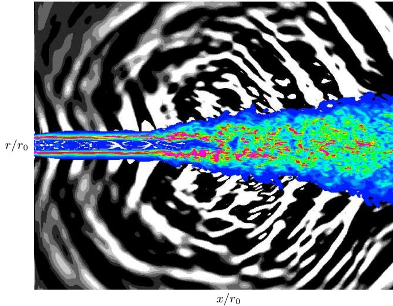
FIGURE 6. Instantaneous dilatation (background) and vorticity magnitude (near image) for a  $M_j = 2.2$  ( $M_d = 2.0$ ) cold jet. The shock cells are visible within the early regions of the jet.  $r_0 = D_j/2$  is the jet radius.
