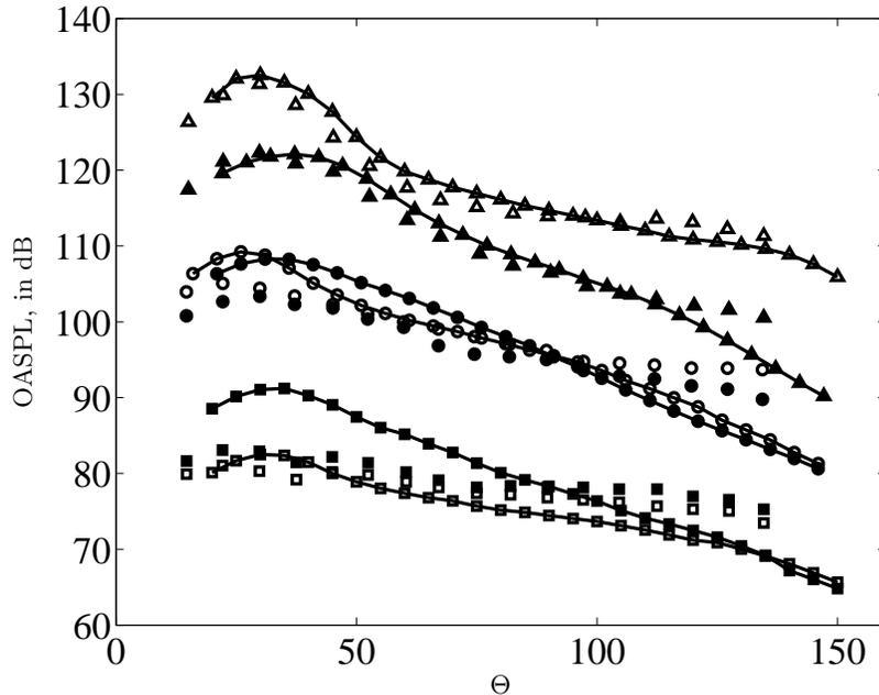
FIGURE 3. Overall sound pressure levels for all six simulated jets at a common distance of  $100D_j$ . Legend:  $-\square-$ , M05TR095;  $-\blacksquare-$ , M05TR176;  $-\circ-$ , M09TR086;  $-\bullet-$ , M09TR270;  $-\triangle-$ , M15TR056;  $-\blacktriangle-$ , M15TR230. Experimental data:  $\square$ , Tanna (M05TR095);  $\blacksquare$ , Tanna (M05TR176);  $\circ$ , Tanna (M09TR086);  $\bullet$ , Tanna (M09TR270);  $\triangle$ , Tanna (M15TR056);  $\blacktriangle$ , Tanna (M15TR230).
