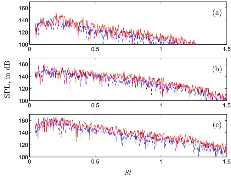
FIGURE 8. Sound pressure levels at  $r/D_j = 6$  corresponding to Fig. 7. Pressure matched jet with  $M_j = 1.95$ , —; imperfectly expanded jet ——. Spectrum measured at (a)  $x/r_0 = 15.7$ , (b)  $x/r_0 = 30.0$ , (c)  $x/r_0 = 44.3$ .
