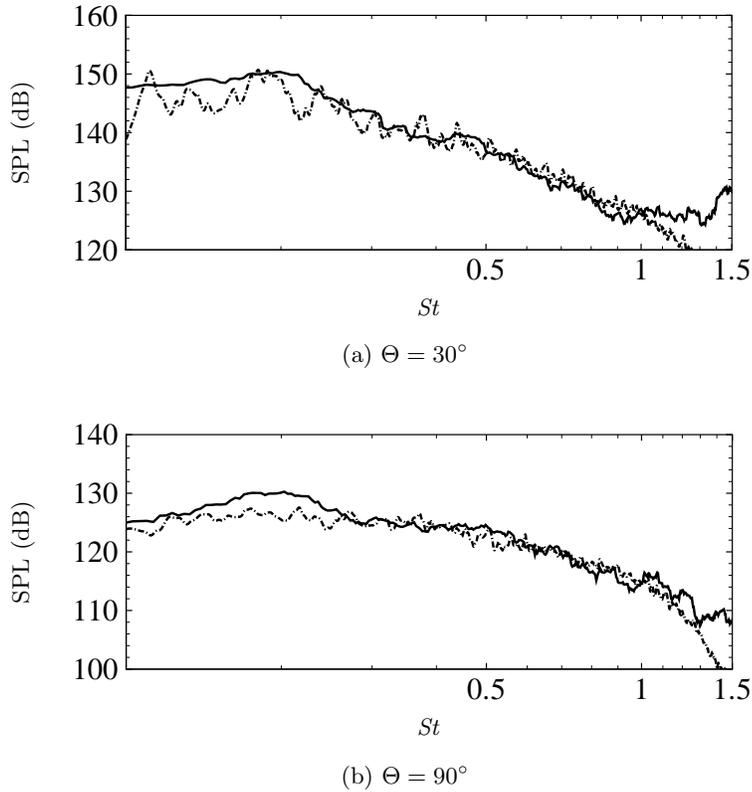
FIGURE 5. Narrowband spectra at  $\mathcal{R} = 30D_j$  for the Mach 1.0 heated jet M15TR230. Lighthill (total), —; Kirchhoff Surface, - - -.
