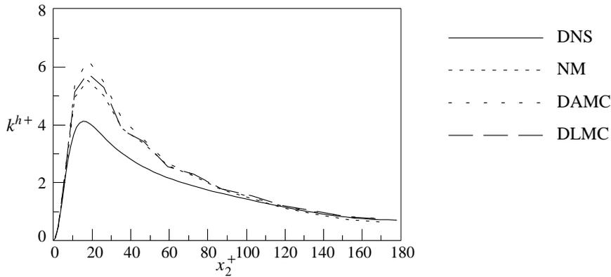
FIGURE 2. Turbulent kinetic energy at  $Re_\tau = 180$
