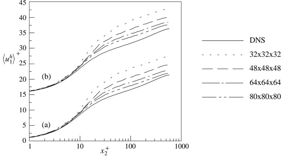
FIGURE 5. Grid refinement effect on mean streamwise velocity at  $Re_\tau = 590$ : (a) DAMC; (b) DLMC (+15)
