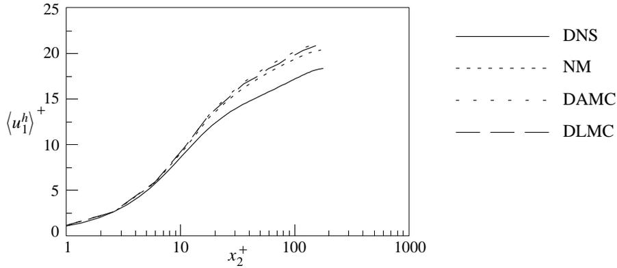
FIGURE 1. Mean streamwise velocity at  $Re_\tau = 180$
