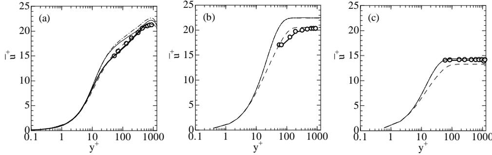
FIGURE 6. Mean streamwise velocity profiles for (a)  $Hr = 0$ , (b)  $Hr = 20.4$ , and (c)  $Hr = 48.9$ : —, CSM; ---, DSM; - - - , SM; -○-, experiment; —, DNS  $Re_\tau = 590$ .
