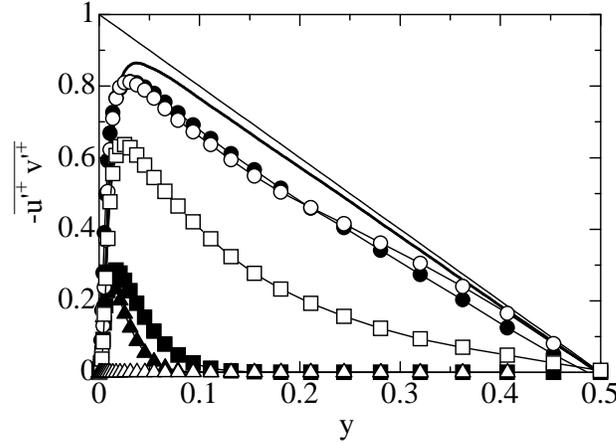
FIGURE 7. Reynolds shear stress profiles for  $Hr = 6.37$  ( $-\circ-$ , CSM;  $-\bullet-$ , SM),  $12.1$  ( $-\square-$ , CSM;  $-\blacksquare-$ , SM), and  $20.4$  ( $-\triangle-$ , CSM;  $-\blacktriangle-$ , SM) :  $-\text{—}$ , DNS  $Re_\tau = 590$ .
