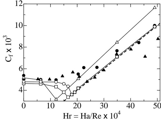
FIGURE 2. Skin friction coefficient  $C_f$  computed with three SGS models ( $-\circ-$ , CSM;  $-\square-$ , DSM;  $-\triangle-$ , SM) as a function of  $Hr = Ha/Re \times 10^4$  at  $Re = 35000$ :  $\bullet$ , the experimental data of Brouillette & Lykoudis (1967) for  $Re_D = 58000$ ;  $\blacktriangle$ , the experimental data of Reed & Lykoudis (1978) for  $Re_D = 53000$ ;  $----$ , the laminar value of the two dimensional solution  $C_f = 2Ha/Re$  (i.e.,  $C_f \times 10^3 = Hr/5$ ).
