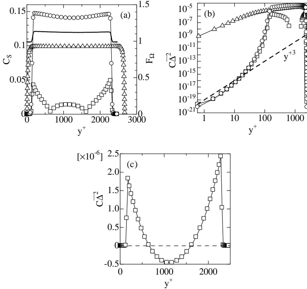
FIGURE 4. Profiles of (a) model parameter  $C_S$  (—,  $F_\Omega$ ), (b) model parameter  $C\bar{\Delta}^2$  near a wall for CSM, DSM, and SM, and (c) model parameter  $C\bar{\Delta}^2$  for DSM, at  $Hr = 48.9$ :  $-\circ-$ , CSM;  $-\square-$ , DSM;  $-\triangle-$ , SM.
