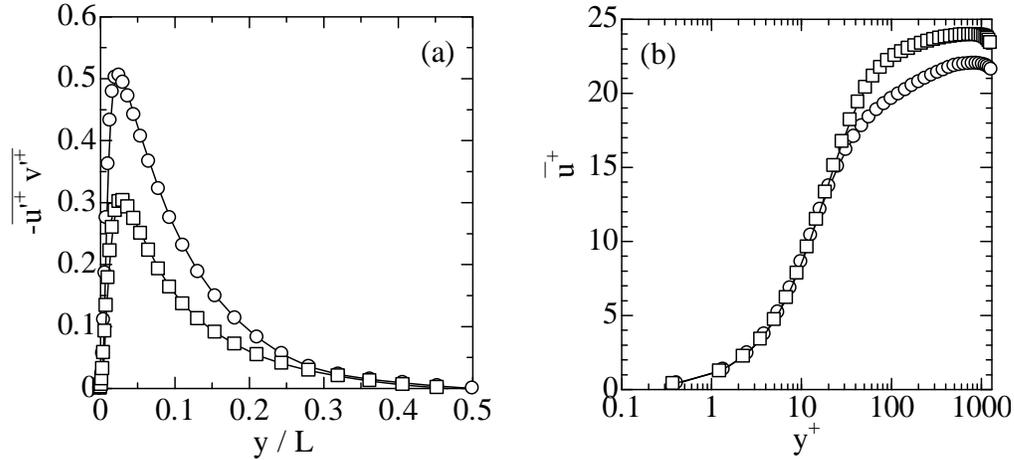
FIGURE 3. Profiles of (a) Reynolds shear stress and (b) mean streamwise velocity computed with CSM and DSM at  $Hr = 15.0$ :  $-\circ-$ , CSM;  $-\square-$ , DSM.
