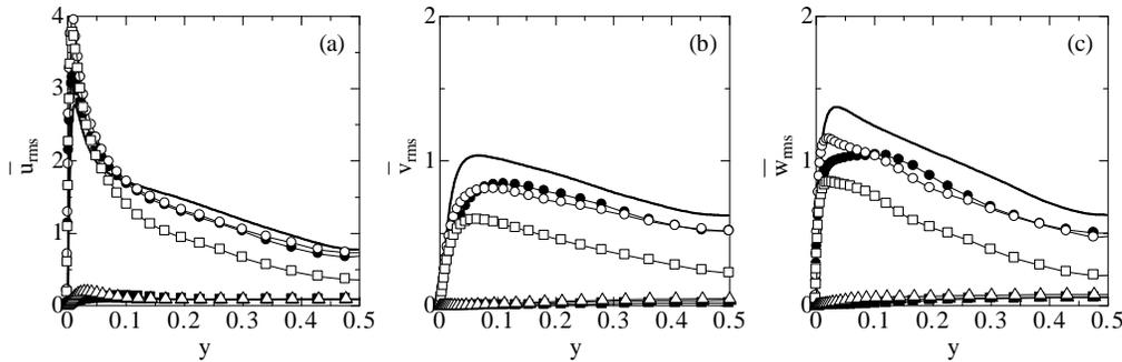
FIGURE 8. Profiles of the rms of velocity fluctuations: (a)  $\bar{u}_{rms}$ , (b)  $\bar{v}_{rms}$ , and (c)  $\bar{w}_{rms}$  for  $Hr = 6.37$  ( $-\circ-$ , CSM;  $-\bullet-$ , SM),  $12.1$  ( $-\square-$ , CSM;  $-\blacksquare-$ , SM), and  $20.4$  ( $-\triangle-$ , CSM;  $-\blacktriangle-$ , SM) :  $-\text{—}$ , DNS  $Re_\tau = 590$ .
