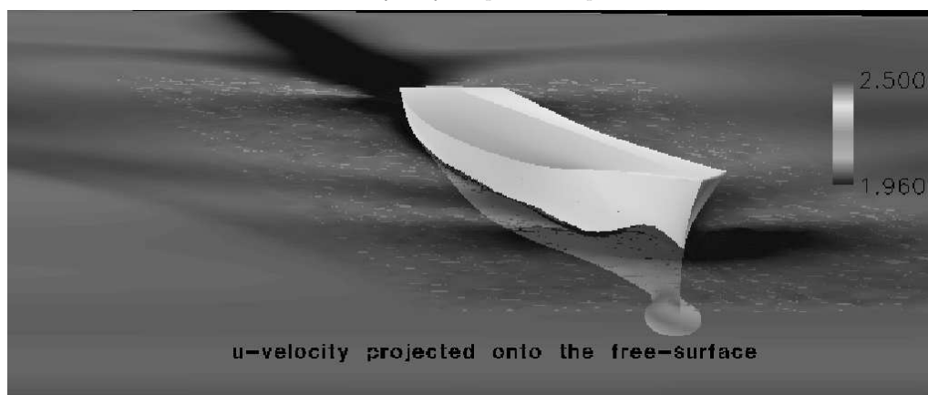
FIGURE 4. Wave pattern on the free surface. The projection of forward velocity onto the free surface is shown.
