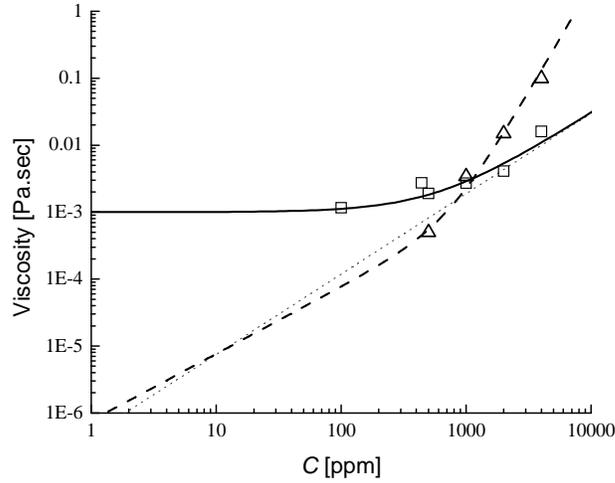
FIGURE 1. Solvent viscosity  $\eta_s$  and polymer viscosity  $\eta_p$  as a function of the concentration of polymer molecules. Experimental data (*WSR301 MI series*) were obtained at the low shear region:  $\square$ ,  $\eta_s$ ;  $\triangle$ ,  $\eta_p$ ; solid line, equation (2.10); dashed line, equation (2.11); dotted line,  $\phi^{1.2}$ .
