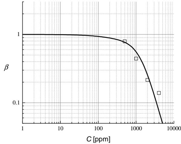
FIGURE 3. The ratio of solvent viscosity to total viscosity,  $\beta = \eta_s/(\eta_s + \eta_p)$ , as a function of the concentration of polymer molecules.  $\square$ , experimental data (*WSR301 MI series*); solid line, prediction from (2.10) and (2.11).
