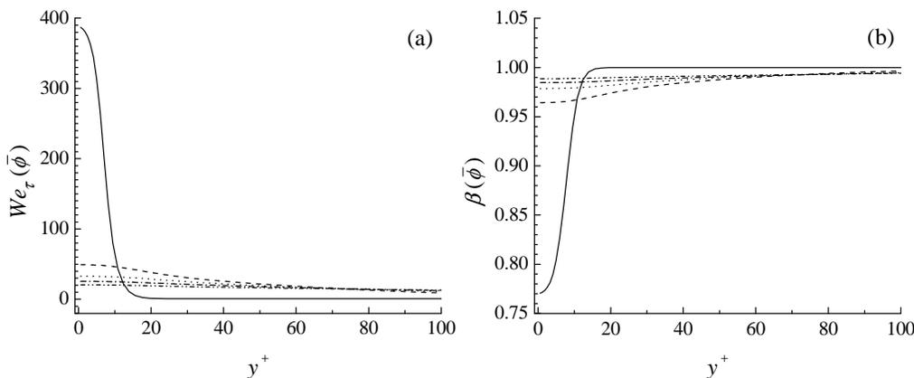
FIGURE 4. Wall-normal distributions of (a)  $We_\tau(\bar{\phi})$  and (b)  $\beta(\bar{\phi})$  at various downstream positions for Case 1: solid line,  $x = 0$ ; dashed line,  $x = 3.4\delta_{in}$ ; dotted line,  $6.8\delta_{in}$ ; dash-dotted line,  $10.2\delta_{in}$ ; dash-dot-dotted line,  $13.6\delta_{in}$ .
