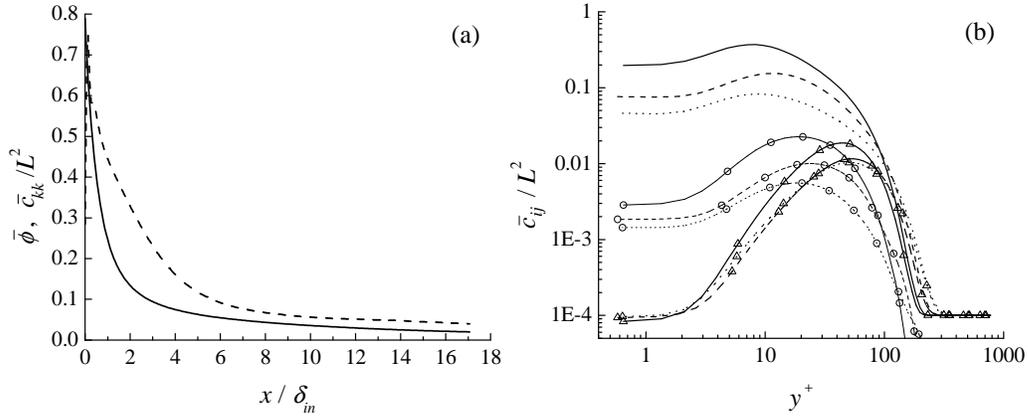
FIGURE 6. Streamwise variations of (a) mean concentration (solid line) and polymer stretching (dashed line) at the wall and (b) wall-normal distribution of  $c_{ij}$  at various downstream positions for Case 1. In (b), solid, dashed and dotted lines indicate the downstream positions of  $x = 3.4\delta_{in}$ ,  $6.8\delta_{in}$  and  $13.7\delta_{in}$ , respectively: lines without symbol,  $c_{xx}$ ; lines with  $\circ$ ,  $c_{xy}$ ; lines with  $\Delta$ ,  $c_{yy}$ .
