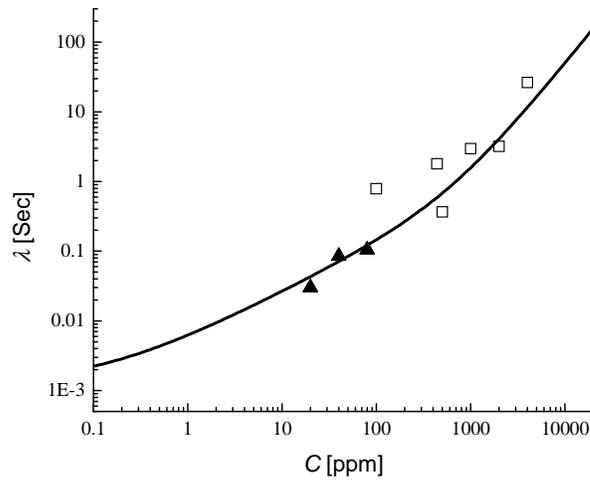
FIGURE 2. Polymer relaxation time  $\lambda$  as a function of the concentration of polymer molecules.  $\square$ , experimental data (*WSR301 MI series*);  $\blacktriangle$ , Kalashnikov's data; solid line, equation (2.12).
