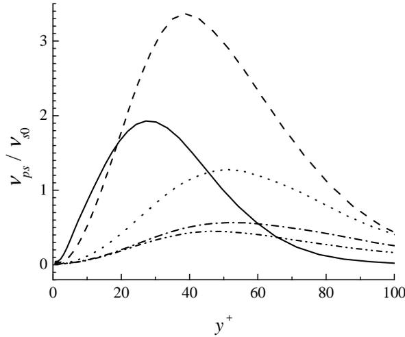
FIGURE 5. Wall-normal distributions of the polymer shear viscosity  $\nu_{ps}$  induced by the polymer stress at various downstream positions in Case 1, where  $\nu_{s0}$  is the kinematic viscosity of pure solvent viscosity: solid line,  $x = 1.7\delta_{in}$ ; dashed line,  $3.4\delta_{in}$ ; dotted line,  $6.8\delta_{in}$ ; dash-dotted line,  $10.3\delta_{in}$ ; dash-dot-dotted line,  $13.7\delta_{in}$ .
