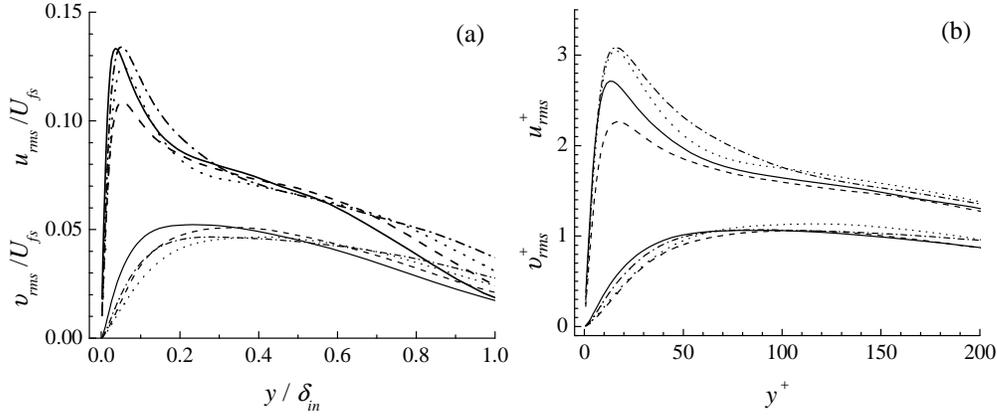
FIGURE 8. The rms values of  $u'$  and  $v'$  normalized with (a) large scale quantities and (b) wall units at various downstream positions in Case 1: solid line, Newtonian; dashed line,  $x = 3.4\delta_{in}$ ; dotted line,  $6.8\delta_{in}$ ; dash-dotted line,  $13.7\delta_{in}$ .
