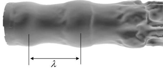
FIGURE 2. Axisymmetric modulation on the liquid surface at the initial stage of the breakup.
