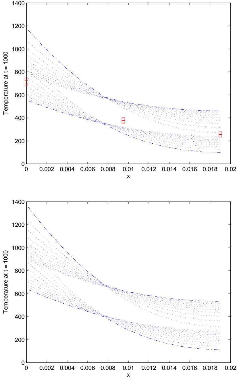
FIGURE 1. 99% confidence interval of  $T$  assuming Gaussian distribution for  $k$  and  $\rho C_p$ . The conditions correspond to  $L = 0.019m$  and  $q = 3000W/m^2$  (top) and to the regulatory assessment  $L = 0.019m$  and  $q = 3500W/m^2$  (bottom).  $\square$ : experimental data - .....: Eq. 2.1 - - - - -: computed confidence bounds.
