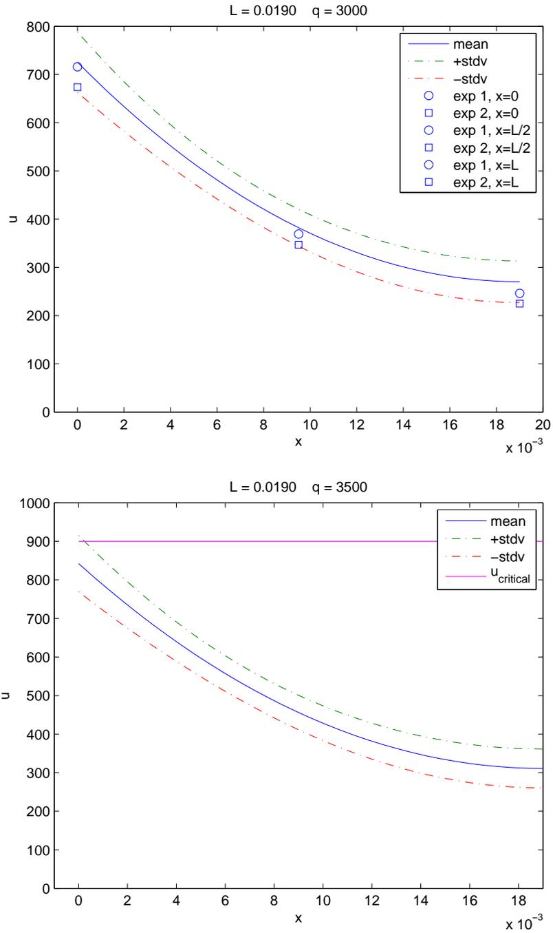
FIGURE 3. Polynomial chaos solution to the 1-D heat conduction problem assuming uniform distribution for  $k$  and  $\rho C_p$ . The conditions correspond to the  $L = 0.019m$  and  $q = 3000W/m^2$  (top) and to the regulatory assessment  $L = 0.019m$  and  $q = 3500W/m^2$  (bottom).  $\square$  : experimental data - .....: Eq. 2.1 - - - - -: computed confidence bounds.
