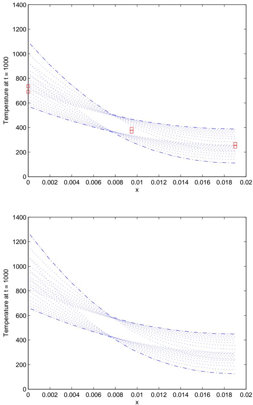
FIGURE 2. 99% confidence interval of  $T$  assuming uniform distribution for  $k$  and  $\rho p_c$ . The conditions correspond to  $L = 0.019\text{m}$  and  $q = 3000\text{W/m}^2$  (top) and to the regulatory assessment  $L = 0.019\text{m}$  and  $q = 3500\text{W/m}^2$  (bottom).  $\square$  : experimental data - .....: Eq. 2.1 - - - - : computed confidence bounds.
