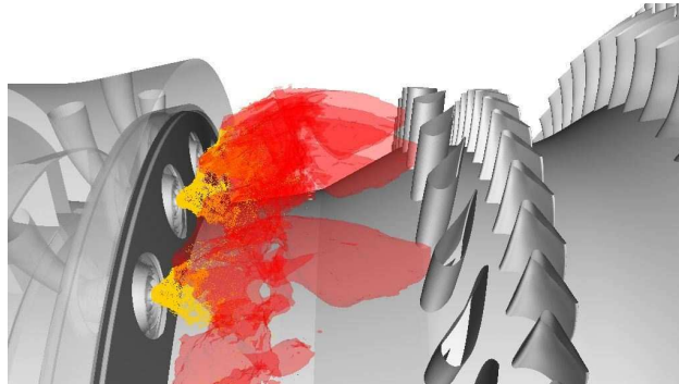
FIGURE 10. Combustor/turbine interface: isosurface of mean temperature.
