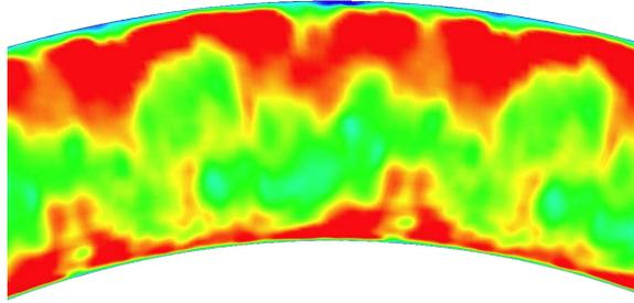
FIGURE 17. Combustor/turbine interface: mean axial velocity.
