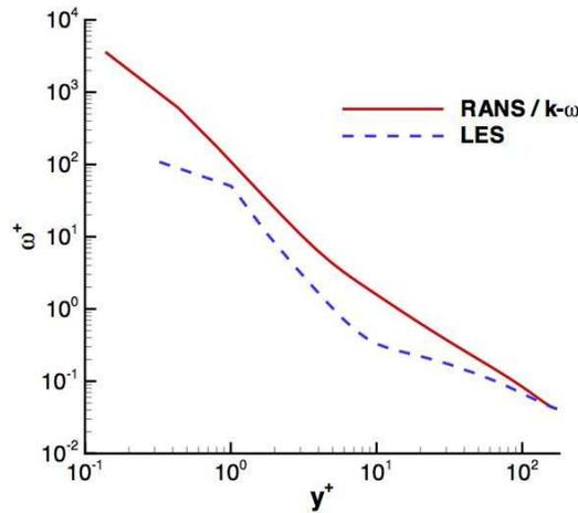
FIGURE 14. Channel flow at  $Re_\tau = 180$ , LES vs. RANS  $k-\omega$  model, specific dissipation rate  $\omega$  computed using  $\varepsilon = \nu \frac{\partial u'_i}{\partial x_k} \frac{\partial u'_i}{\partial x_k}$ .
