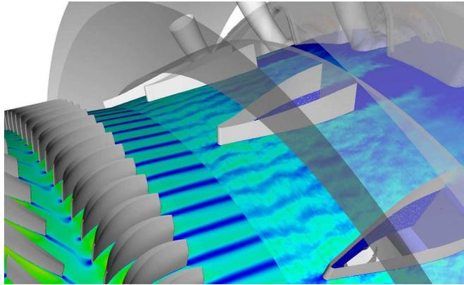
FIGURE 1. Compressor and combustor: RANS and LES axial velocity, mid-passage.
