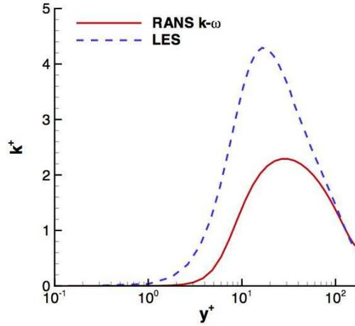
FIGURE 13. Channel flow at  $Re_\tau = 180$ , LES vs. RANS  $k-\omega$  model, turbulent kinetic energy  $k$ .
