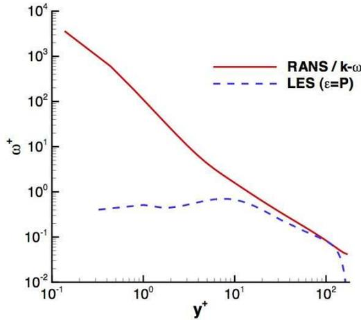
FIGURE 15. Channel flow at  $Re_\tau = 180$ , LES vs. RANS  $k-\omega$  model, specific dissipation rate  $\omega$  computed using  $\varepsilon = P$ .
