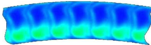
FIGURE 3. Compressor/combustor interface: turbulent kinetic energy from RANS.
