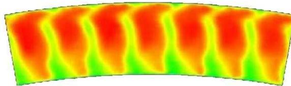
FIGURE 7. Compressor/combustor interface: mean axial velocity.
