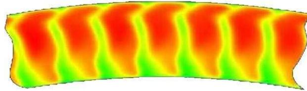
FIGURE 2. Compressor/combustor interface: axial velocity from RANS.
