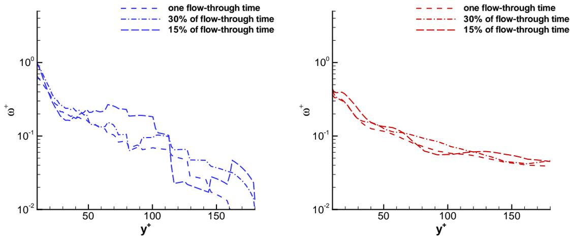
FIGURE 16. Channel flow at  $Re_\tau = 180$ , LES, specific dissipation rate  $\omega$  in the logarithmic layer, computed using  $\varepsilon = \nu \frac{\partial u'_i}{\partial x_k} \frac{\partial u'_i}{\partial x_k}$  (left) and  $\varepsilon = P$  (right) with the statistics for  $\varepsilon$  and  $k$  over very short time windows.
