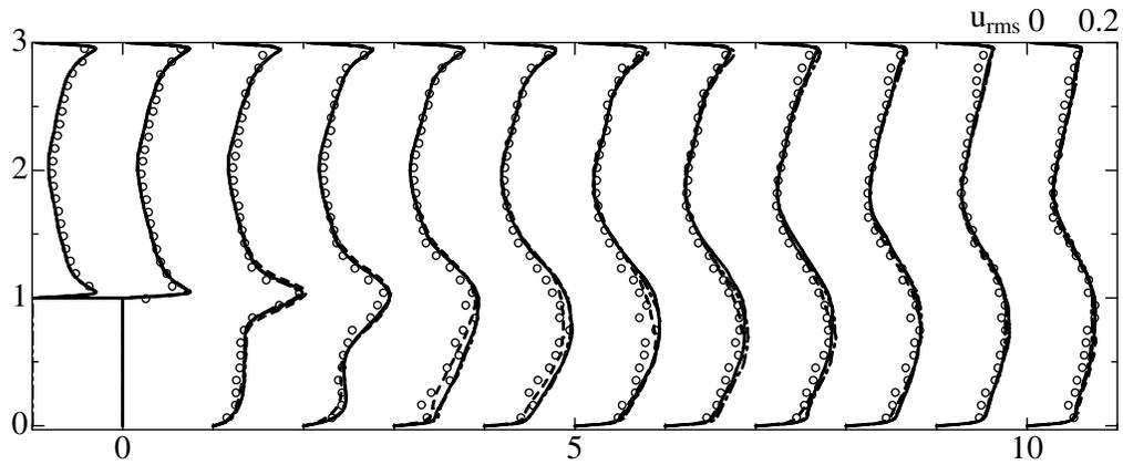
FIGURE 3. Streamwise rms velocity profiles. —, CSM; —·—, DSM; ----, no model;  $\circ$ , experimental data by Kasagi and Matsunaga (1995).
