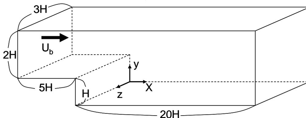
FIGURE 1. Computational domain for a backward-facing step.
