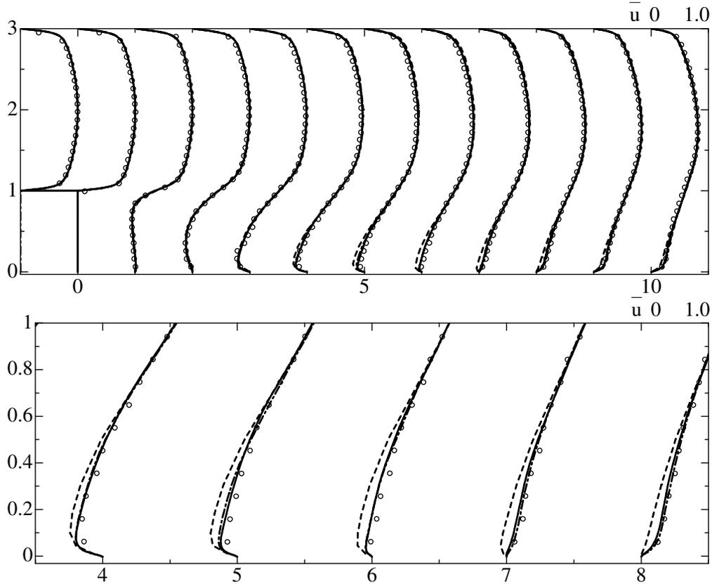
FIGURE 2. Streamwise mean velocity profiles; (upper figure): inlet  $\leq x \leq 10$ ,  $0 \leq y \leq 3$ ; (lower figure):  $4 \leq x \leq 8$ ,  $0 \leq y \leq 1$ . —, CSM; —·—, DSM; ----, no model;  $\circ$ , experimental data by Kasagi and Matsunaga (1995).
