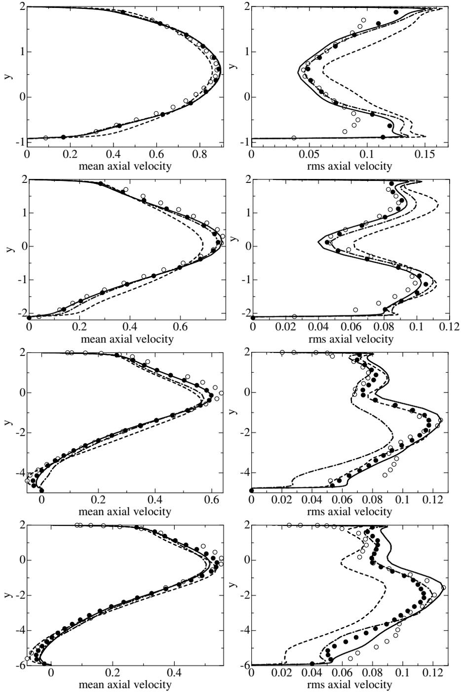
FIGURE 8. Streamwise profiles of mean (left column) and rms (right column) velocities at  $x = 5.18, 11.96, 27.1,$  and  $33.86$  from top to bottom. —, CSM; ---, DSM; ···, no model; ●, fine DSM; ○, experimental data by Buice and Eaton (1997).
