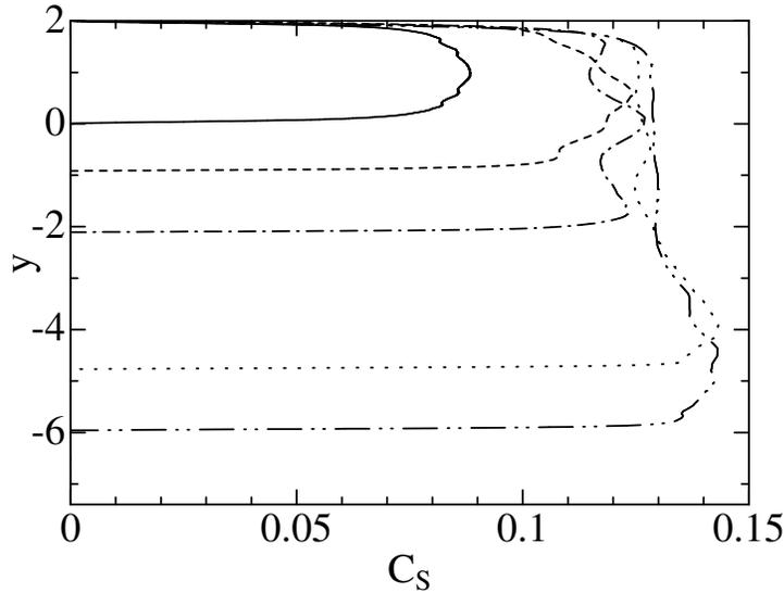
FIGURE 9. Profiles of Smagorinsky constant  $C_s = \sqrt{C}$  for the CSM. —,  $x = -5$ ; ----, 5.18; — · —, 11.96; ·····, 27.1; - - - -, 33.86.
