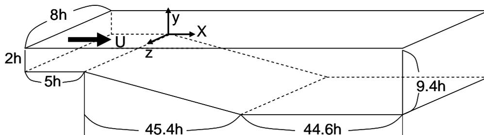
FIGURE 7. Computational domain for an asymmetric plane diffuser.
