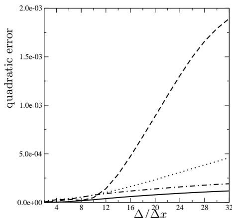
FIGURE 3. Evolution of the quadratic errors of the scale similarity and dynamic Smagorinsky-type models and their associated irreducible error with the filter width.  $\langle (z_v - \langle z_v | \phi_1 \rangle)^2 \rangle$  — ;  $\langle (z_v - z_{v,DM})^2 \rangle$  - - - - ;  $\langle (z_v - \langle z_v | \phi_2 \rangle)^2 \rangle$  - · - · ;  $\langle (z_v - z_{v,SS})^2 \rangle$  ····· .
