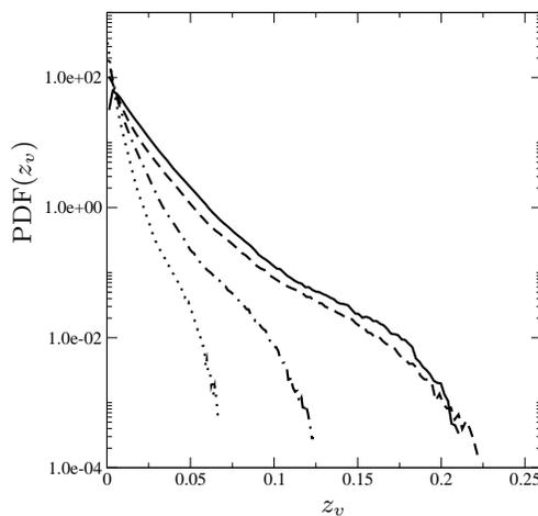
FIGURE 12. PDF of the subfilter scalar variance for  $\Delta/\Delta x = 14$ .  $z_v$  — ;  $z_{v,DM}$   $\cdots$  ;  $z_{v,o2}$   $-\cdot-$  ;  $z_{v,NM}$   $- - -$  .
