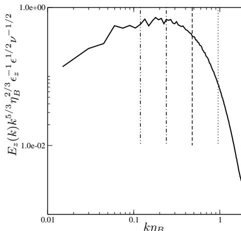
FIGURE 2. Compensated scalar variance spectrum with the location of filters used in this work (see Fig. 1 for legend).
