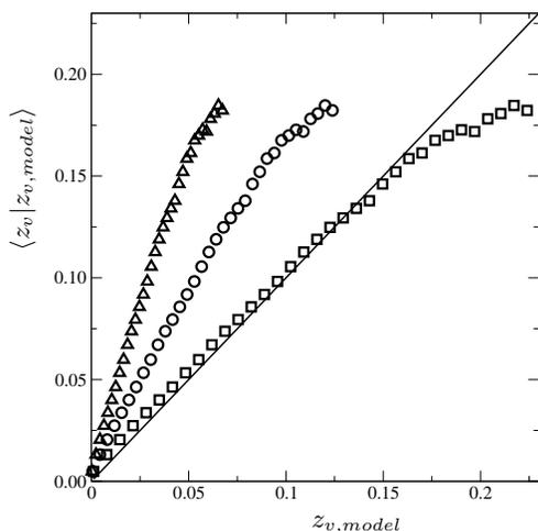
FIGURE 11. Plot of  $\langle z_v | z_{v,model} \rangle = f(z_{v,model})$  for  $\Delta/\Delta x = 14$ ;  $z_{v,DM}$   $\triangle \triangle \triangle$ ;  $z_{v,o2}$   $\circ \circ \circ$ ;  $z_{v,NM}$   $\square \square \square$ ;  $y = x$  — .
