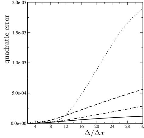
FIGURE 10. Evolution of the quadratic errors of the models  $z_{v,DM}$ ,  $z_{v,o2}$  and  $z_{v,NM}$  and the associated irreducible error with the filter width.  $\langle(z_v - \langle z_v | \phi_1 \rangle)^2\rangle$  ———;  $\langle(z_v - z_{v,DM})^2\rangle$  ·····;  $\langle(z_v - z_{v,o2})^2\rangle$  - - - -;  $\langle(z_v - z_{v,NM})^2\rangle$  ———.
