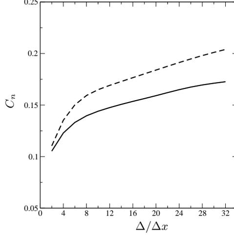
FIGURE 9. Model constant computing following both ways given in Eqs. 3.25 and 3.26.  $C_n = \langle L_n M_n \rangle / \langle M_n M_n \rangle$  — ;  $C_n = \langle L_n \rangle / \langle M_n \rangle$  - - - .
