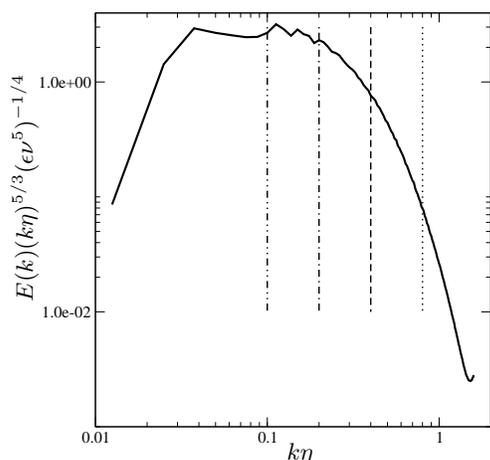
FIGURE 1. Compensated kinetic energy spectrum with the location of filters used in this work.  $\Delta/\Delta x = 2$   $\cdots\cdots$ ;  $\Delta/\Delta x = 4$   $-\cdot-\cdot-$ ;  $\Delta/\Delta x = 8$   $-\cdot-\cdot-$ ;  $\Delta/\Delta x = 16$   $-\cdot-\cdot-$ .
