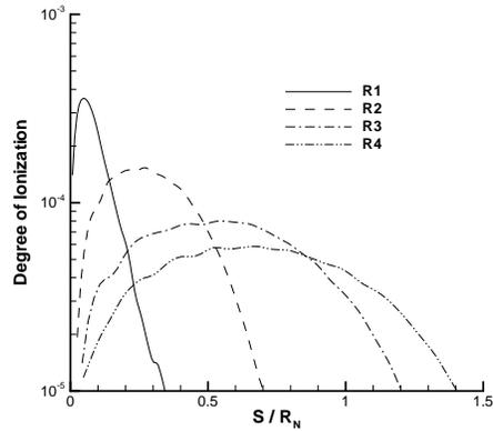
FIGURE 16. Profiles of ionization degree as a function of distance from the surface along the four reflectometer lines.
