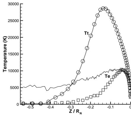
FIGURE 7. Temperature profiles along the stagnation streamline for the RAM-C II nose cap region simulation: lines=reduced electron mass.
