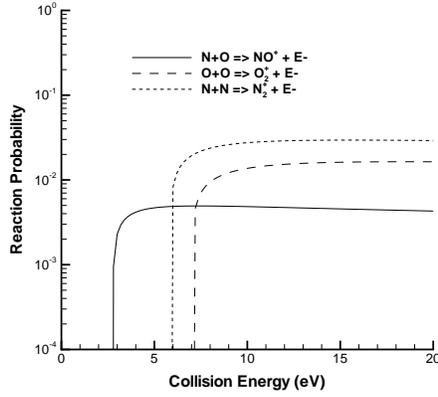
FIGURE 2. Probability of associative ionization as a function of collision energy obtained with the TCE model.
