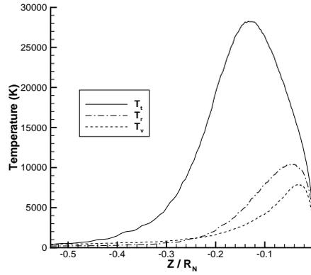
FIGURE 6. Temperature profiles along the stagnation streamline for the RAM-C II nose cap region simulation.
