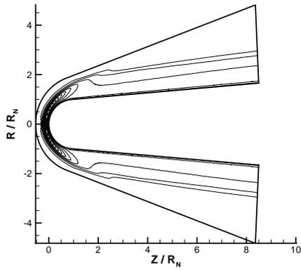
FIGURE 11. Contours of translational temperature (K) for the full-scale RAM-C II simulation.
