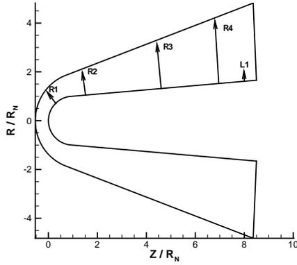
FIGURE 1. Computational domain for flow around the RAM-C II vehicle including the locations of the reflectometers (R1–R4) and the rake of Langmuir probes (L1).
