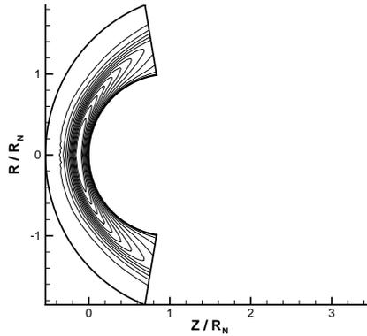
FIGURE 4. Contours of translational temperature (K) for the RAM-C II nose cap region simulation.
