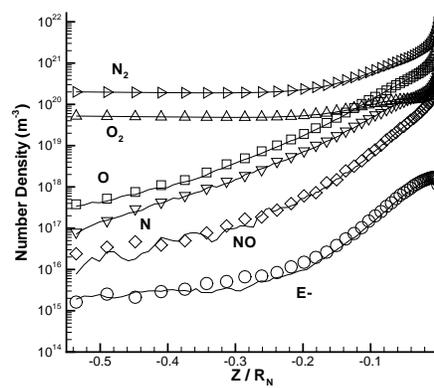
FIGURE 8. Species number density profiles along the stagnation streamline for the RAM-C II nose cap region simulation: lines=reduced electron mass.
