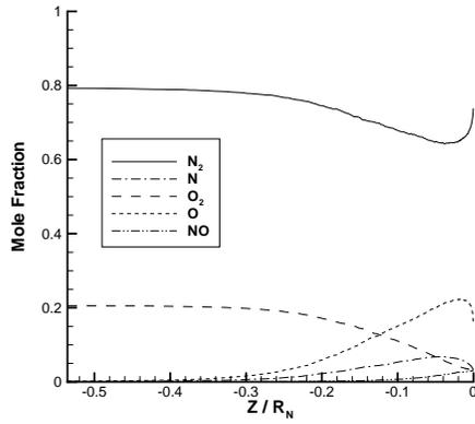
FIGURE 5. Mole fraction profiles along the stagnation streamline for the RAM-C II nose cap region simulation.
