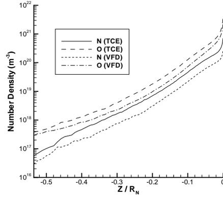
FIGURE 14. Profiles of atom number density obtained along the stagnation streamline with two different chemistry models.
