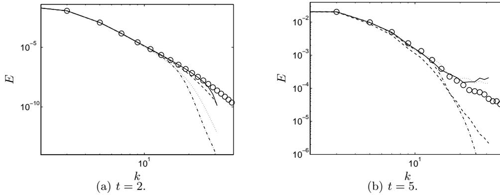
FIGURE 3. Velocity spectra of inviscid Taylor-Green vortex on  $64^3$  grid. Split forms of eighth- (S8, solid) and second- (S2, dotted) order accuracy, with eighth-order dissipation (S8D8, dash-dotted), and seventh-order WENO (W7, dashed). Converged spectrum on  $256^3$  (circles).
