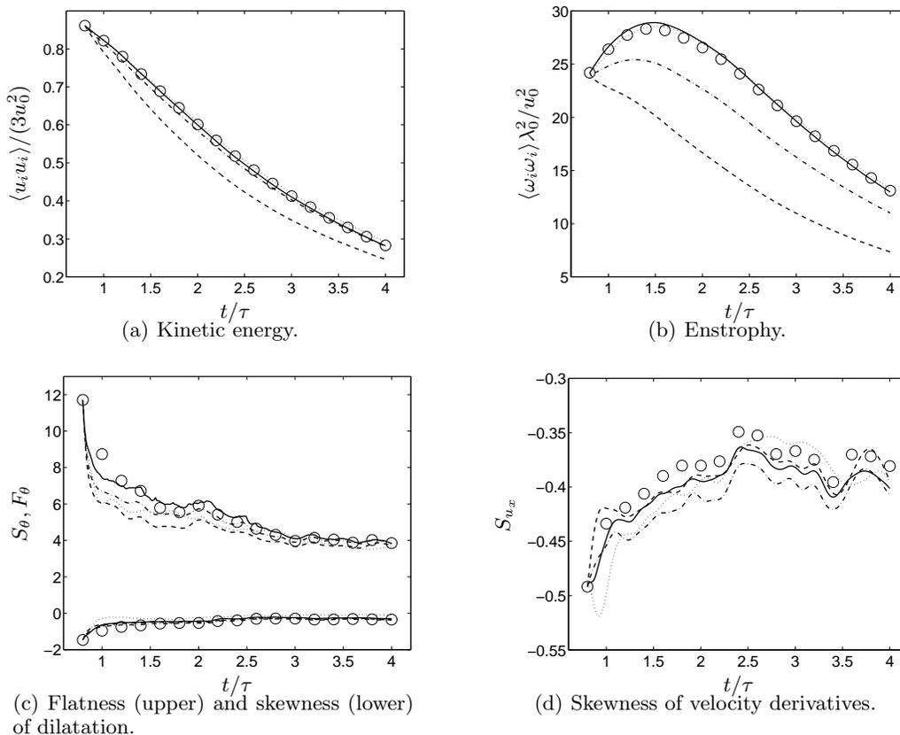
FIGURE 5. Isotropic turbulence on  $64^3$  grid, starting from filtered field at  $t/\tau = 0.8$ . Hybrid methods with eighth- (H8, solid) and second- (H2, dotted) order central schemes, with eighth-order dissipation (H8D8, dash-dotted), and seventh-order WENO (W7, dashed). Filtered  $256^3$  results (circles).
