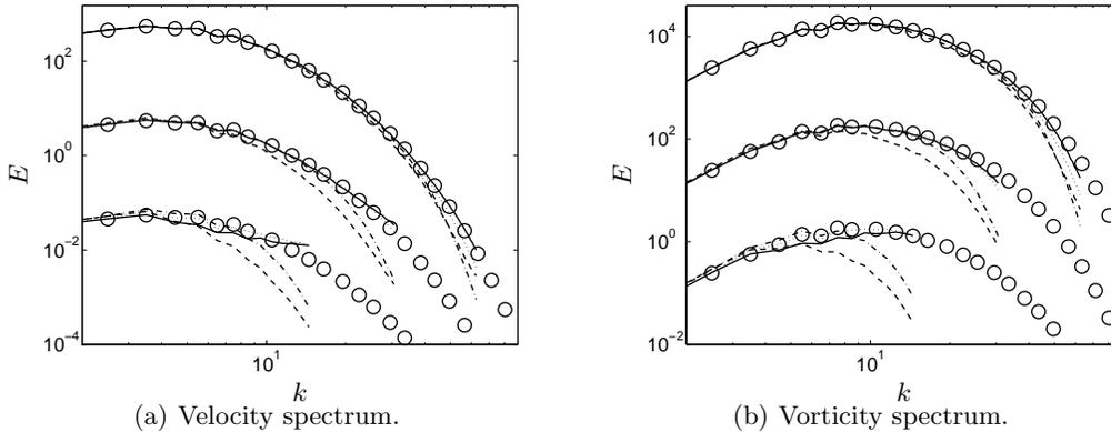
FIGURE 6. Spectra of isotropic turbulence at  $t/\tau = 4$ . Hybrid methods with eighth- (H8, solid) and second- (H2, dotted) order central schemes, with eighth-order dissipation (H8D8, dash-dotted), and seventh-order WENO (W7, dashed). Converged spectrum on  $256^3$  grid (circles). Grids from bottom to top (with offset):  $32^3$ ,  $64^3$  and  $128^3$ .
