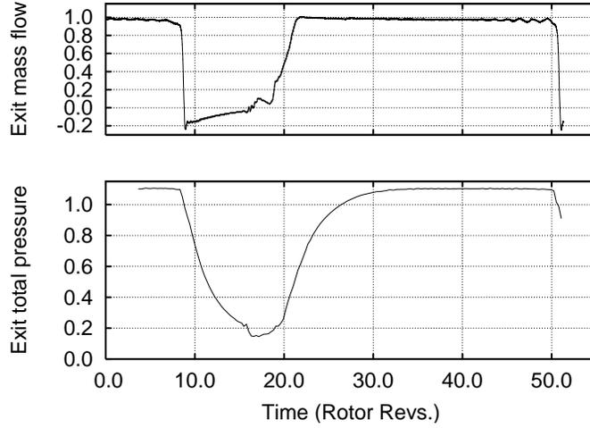
FIGURE 4. Surge cycle. Top: compressor exit mass flow rate. Bottom: combustion chamber pressure.
