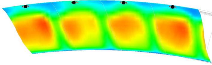
(a) 5RB exit axial velocity contour. Black dots denote points where the velocities are plotted.
