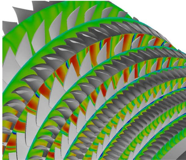
FIGURE 7. Axial velocity contours at time  $T_3$ .
