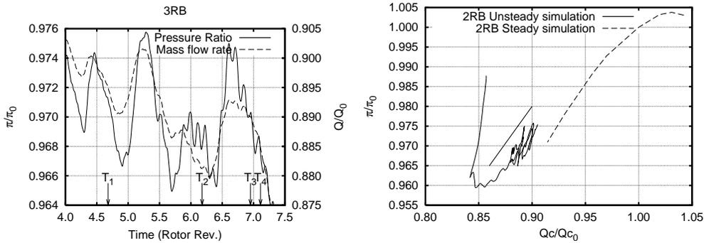
(a) Histories of pressure ratio & mass flow rate. (b) Characteristic curve.
