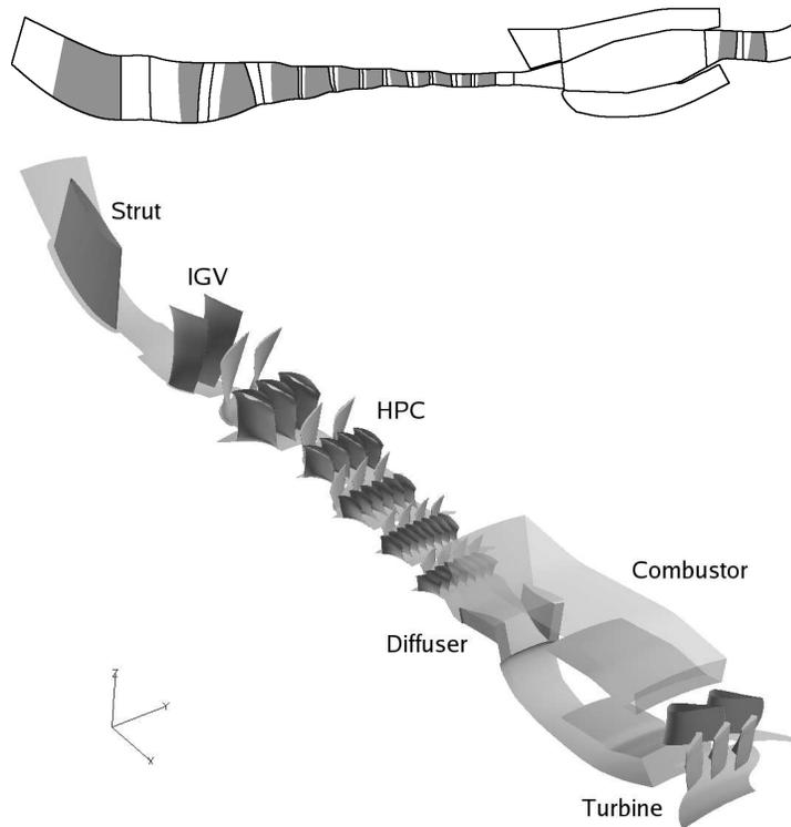
FIGURE 1. Geometry of the computational model.
