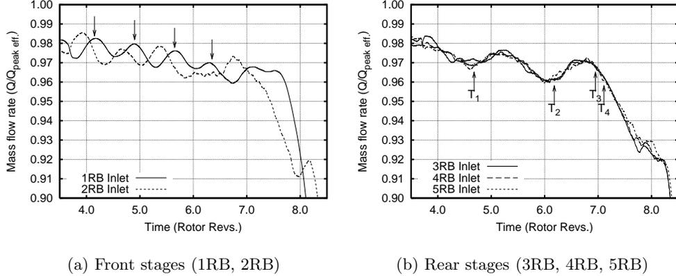
FIGURE 5. Mass flow at each stage.
