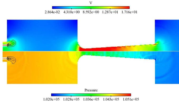
FIGURE 6. Snapshots of the velocity (top) and pressure (bottom) after 5.3 ms. Mixture fraction contours are superimposed, 2-D results.
