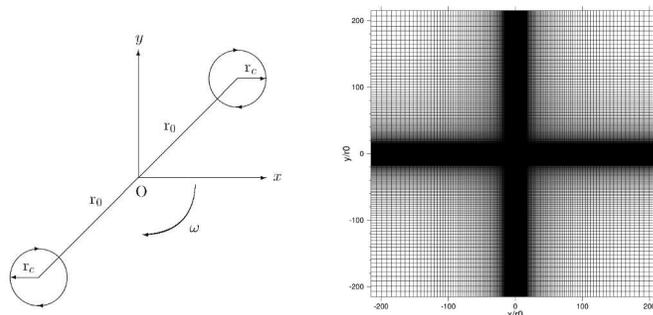
FIGURE 1. Dual vortices test case. Left: Schematic view of the configuration. Right: 2-D mesh.
