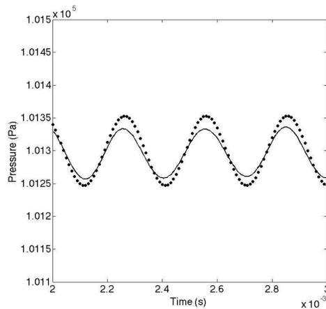
FIGURE 3. Pressure traces at  $r/\lambda = 0.55$ , with an angle of  $45^\circ$  off the axis. Results of the simulation (—), analytical response obtained from Eq. (3.1) (●).
