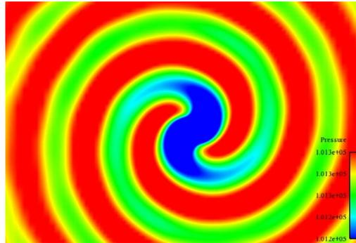
FIGURE 2. Snapshot of the pressure field illustrating the quadrupole spiral pattern.
