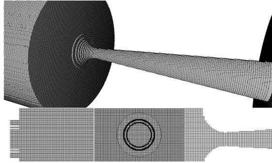
FIGURE 5. The 3-D structured mesh used for the simulations.  $\Delta y$  and  $\Delta z$  are kept constant and equal to  $5 \cdot 10^{-4}$  m.
