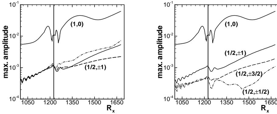
FIGURE 10. Left: same as Fig. 7 (left), but results for two different values of the phase difference at the location of their respective disturbance strip  $\Delta\Psi = 0$  (—) and  $\Delta\Psi = \pi/2$  (- -). The linear evolution is given for reference (- · -). Right: same as Fig. 7 (left), but results for three different spanwise wave length as given by the respective labels in the diagram.
