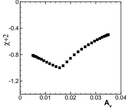
FIGURE 9. Response curve for the non-linear case, i.e.,  $\chi$  at  $R_x = 1550$  for a roughness height  $h_R = 0.125$  as a function of primary amplitude.
