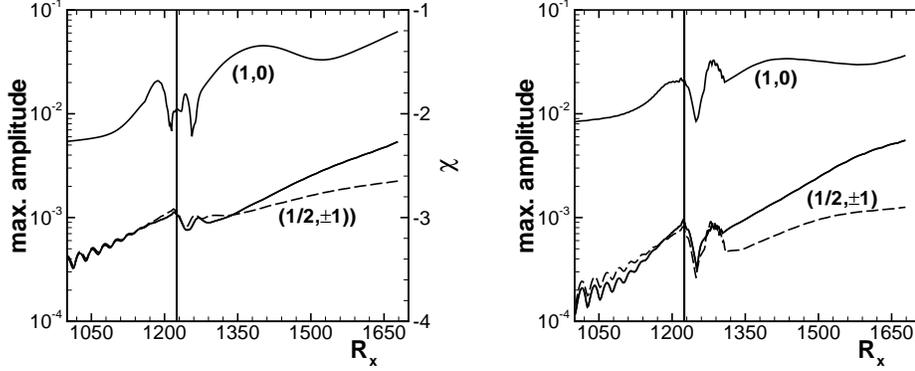
FIGURE 7. Amplitudes  $\hat{a}_{(h,k)}^{max}$  for  $h_R = 0.125$  with  $A_v^{2-D} = 0.035$  (—) and  $A_v^{2-D} = 0.0$  (---). Quantities  $a = u$  (left) and  $a = \rho$  (right).
