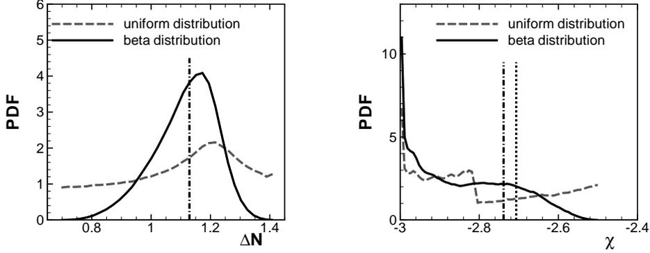
FIGURE 11. Left: PDFs for  $\Delta N$  at  $R_x = 1750$  for the linear case using 34 bins. The vertical line (---) marks the deterministic value for  $h_R = 0.1$ . Right: PDFs for  $\chi$  at  $R_x = 1550$  for the non-linear case using 68 bins. The vertical lines mark the value for linear disturbance evolution,  $A_v^{2-D} = 0.0$ , for a flat plate (---) and for  $h_R = 0.125$  (.....).
