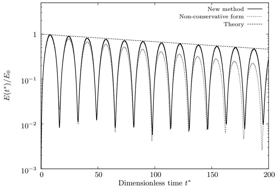
FIGURE 4. Decay of the total energy of an oscillating viscous drop (density ratio: 1000).
