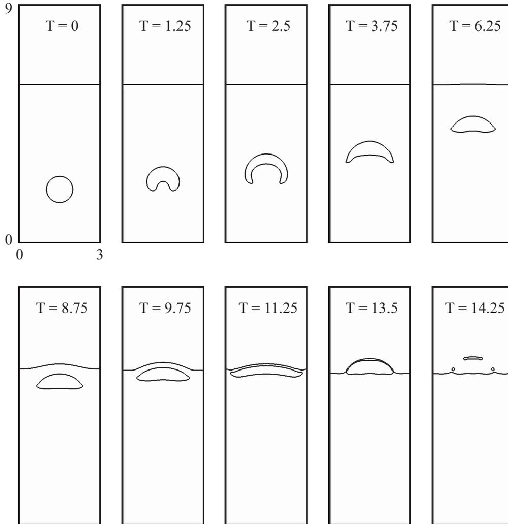
FIGURE 5. Rise, deformation, and burst of a two-dimensional bubble in a liquid pool (density ratio: 1000).
