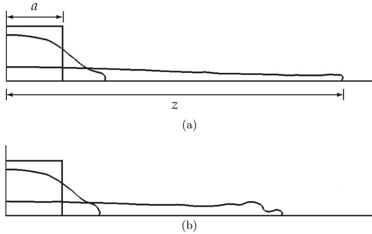
FIGURE 2. Collapse and spread of a water column in air simulated by (a) the new method and (b) the non-conservative formulation of the flow equation (density ratio: 815).
