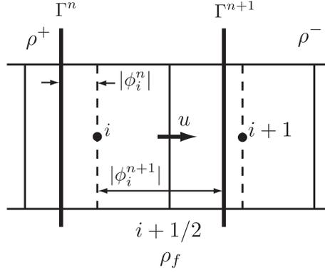
FIGURE 1. Calculation of flux density across surface  $i$  from the signed distance function  $\phi$  at two consecutive time levels  $n$  and  $n + 1$ .
