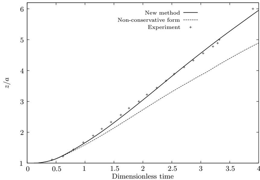
FIGURE 3. Non-dimensional front position of collapsing water columns in air, shown in Fig. 2, versus dimensionless time (density ratio: 815).
