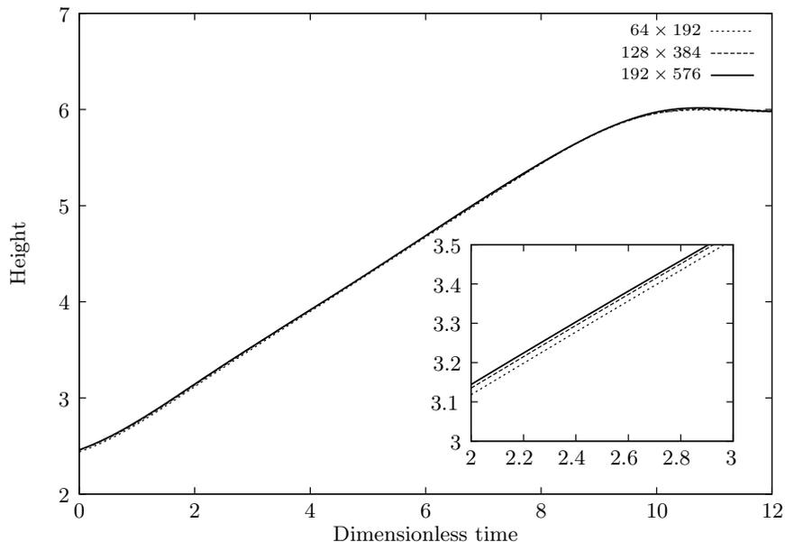
FIGURE 6. Bubble height versus dimensionless time for different mesh resolutions.
