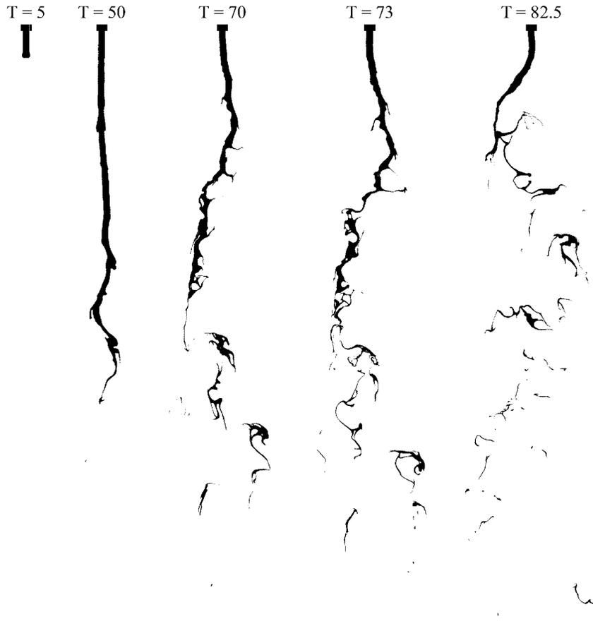
FIGURE 7. Breakup of ethanol in shear air flow (density ratio: 650).
