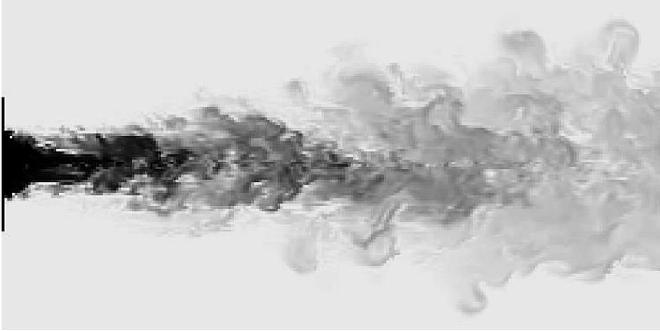
FIGURE 1. Density field from helium plume simulation at  $Re_D = 3000$  and  $Ri = 76$  showing Rayleigh-Taylor unstable bubbles near plume base. The graphic shows the instant near the beginning of a puff cycle, with previous puff already rising from the plume base. Grayscale value black (white) is helium (air). Axial direction (*left to right*) is opposed to gravity vector.
