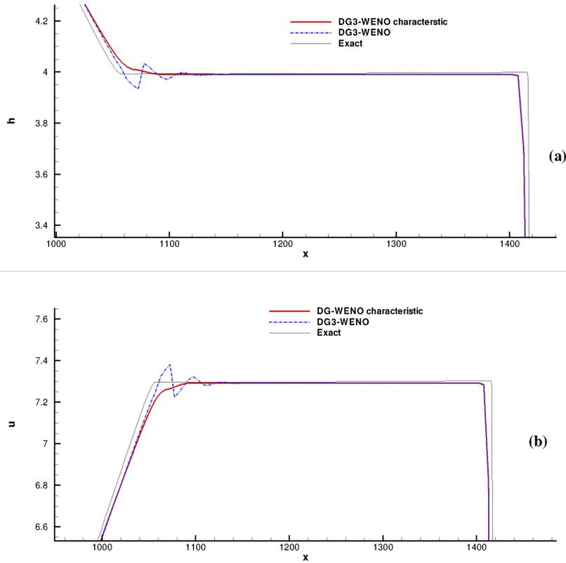
FIGURE 5. The water depth (a) and flow velocity (b) predicted for 1D dam-break problem (400 grid points)
