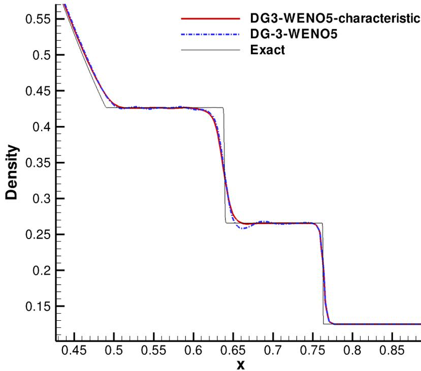
FIGURE 1. Density at time 0.15 for the Sod shock tube problem
