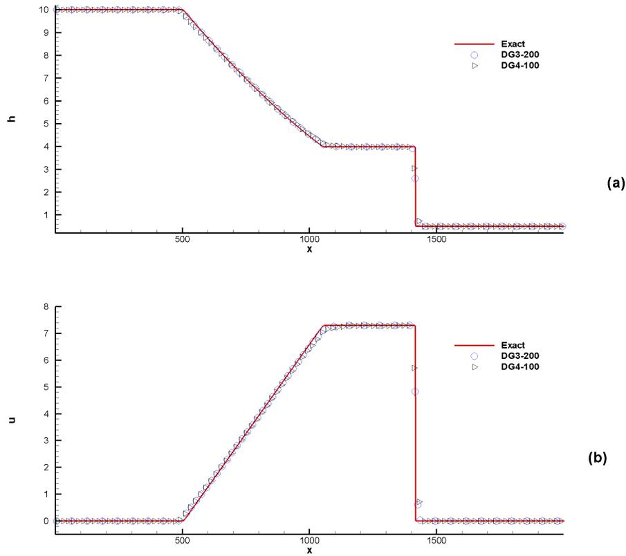
FIGURE 4. The water depth (a) and flow velocity (b) predicted for the 1D dam-break problem
