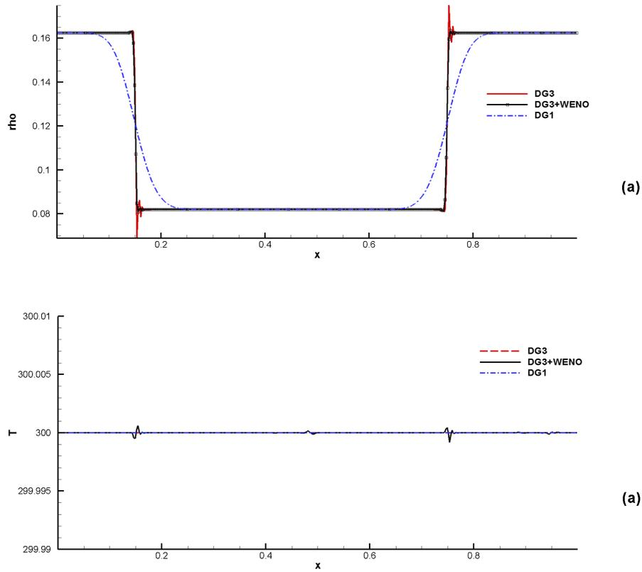
FIGURE 6. Density (a) and temperature (b) at time 0.0015s predicted for binary mixture of hydrogen and helium.
