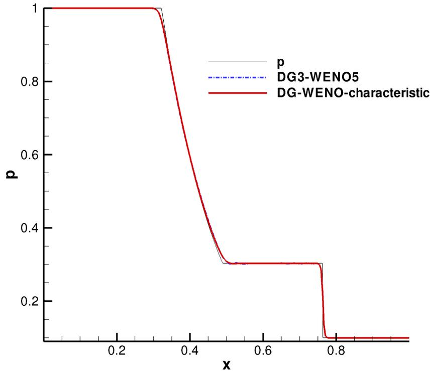
FIGURE 3. Pressure at time 0.15 for Sod shock tube problem
