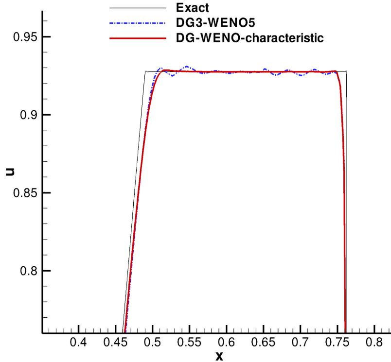
FIGURE 2. Velocity at time 0.15 for Sod shock tube problem
