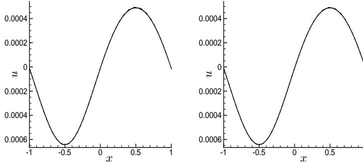
FIGURE 1. Small perturbation of velocity results by central filter schemes:  $\epsilon = 10^{-3} \times \sin(\pi x)$ . *Left*: CEN6WENO5fi 50 points; *Right*: CEN8WENO7fi 50 points (Central filter schemes: dash-dot; Reference 1200 points: solid).
