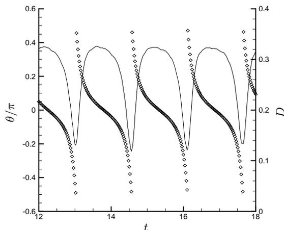
FIGURE 5. Inclination angle  $\theta$  and deformation parameter  $D$  of a tumbling vesicle:  $\diamond$  is for  $\theta$  and  $\text{—}$  is for  $D$ . The simulation is at  $v = 0.9$ ,  $\lambda = 10$  and  $\chi = 8$ .
