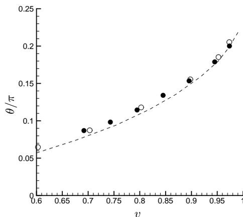
FIGURE 3. The inclination angle of steady-state tank-treading vesicles. The viscosity contrast  $\lambda = 1$ : ● is our simulation results at  $\chi = 9$ , ○ is by Kraus at  $\chi = 10$  Kraus *et al.* (1996), and the dashed line is the theoretical prediction in Kraus *et al.* (1996).
