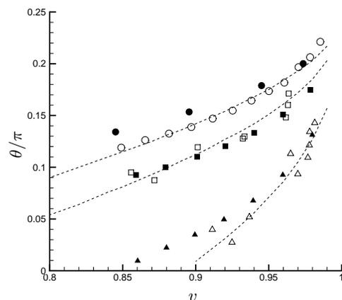
FIGURE 4. The inclination angle of vesicles at three different viscosity ratios: ● for  $\lambda = 1$ , ■ for  $\lambda = 2.7$ , and ▲ for  $\lambda = 5.4$ . The solid symbols are by our simulation; the empty symbols are from the experiment measurements of Kantsler & Steinberg (2005), and the dashed lines are the power law fitting of Kantsler.
