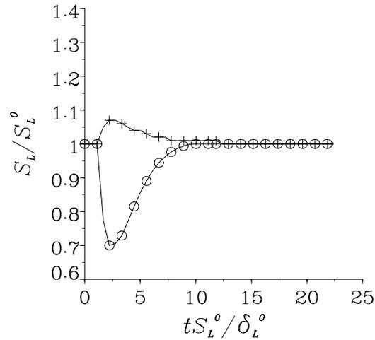
FIGURE 3. Time series of flame speed at the leading edge (+) and flame trough (o) when exposed to a variable mixture fraction. When the mixture fraction is first felt by the flame, the leading edge's flame speed increases, and the trough's flame speed decreases. After some time, both converge to the premixed planar flame speed,  $S_L^0$ . The values of  $Z$  in the troughs are 0.44 and 0.56.
