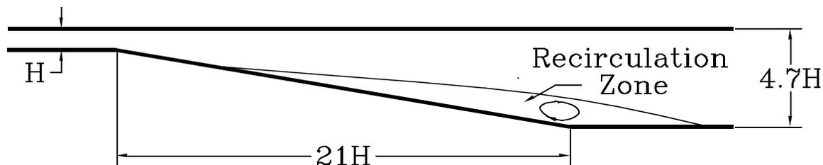
FIGURE 1. Plane diffuser.
