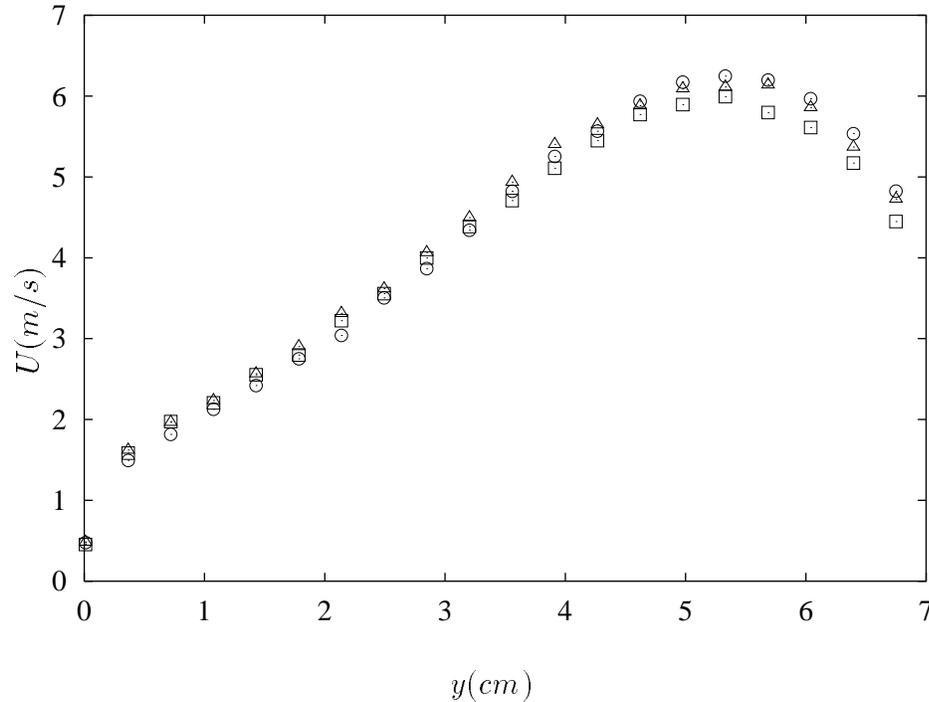
FIGURE 3. Mean-velocity profiles at  $x/\delta = 59$ :  $\circ$ , centerline;  $\triangle$ , near end-wall;  $\square$ , far end-wall.
