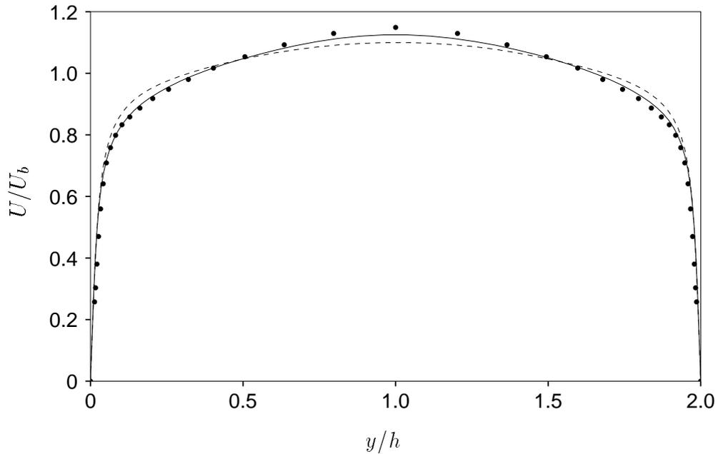
FIGURE 2. Comparison of inflow profiles with experiments: ---- Inlet condition for Run A ( $\Delta x_{in}^+ = 100$ ); — Inlet condition for Run B ( $\Delta x_{in}^+ = 50$ ); • Experimental data by Buice & Eaton (1996).
