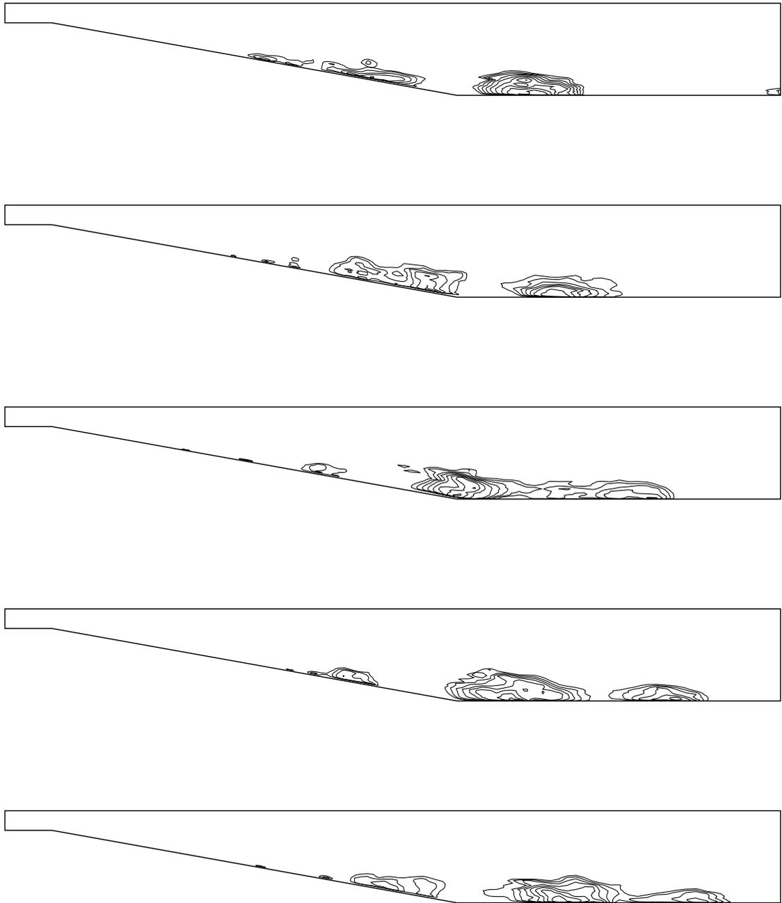
FIGURE 6. Contour line of negative streamwise velocity averaged in the spanwise direction. Time increment among frames is approximately  $30U_b/h$ .
