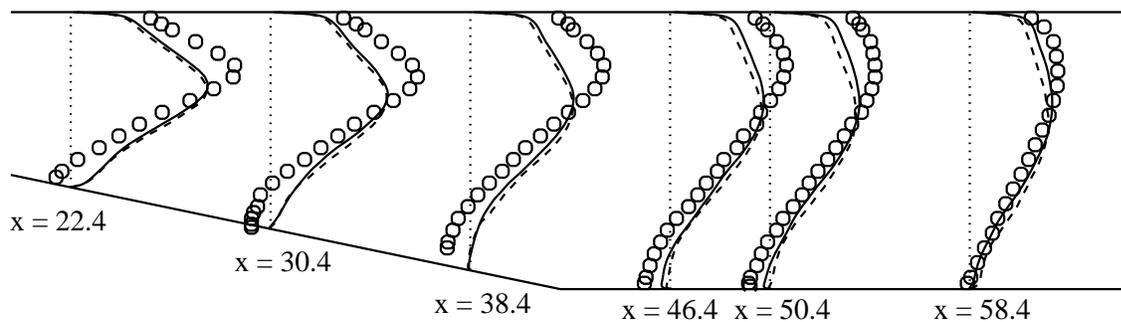
FIGURE 1. Mean velocity profiles  $x + 10U/U_b$  in the exit section of the diffuser. Effect of spanwise resolution. — Run A ; ---- Kaltenbach (1994);  $\circ$  Experimental data by Obi *et al.* (1993).
