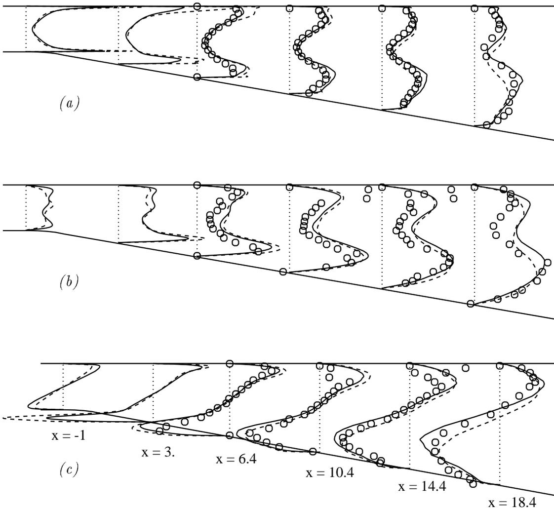
FIGURE 5. Variances  $x + 150\overline{uu}/U_b^2$  (a),  $x + 500\overline{vv}/U_b^2$  (b) and shear stress  $x + 750\overline{uv}/U_b^2$  (c) in the first half of diffuser. — Run B ---- Kaltenbach (1994); o Obi *et al.* (1993).
