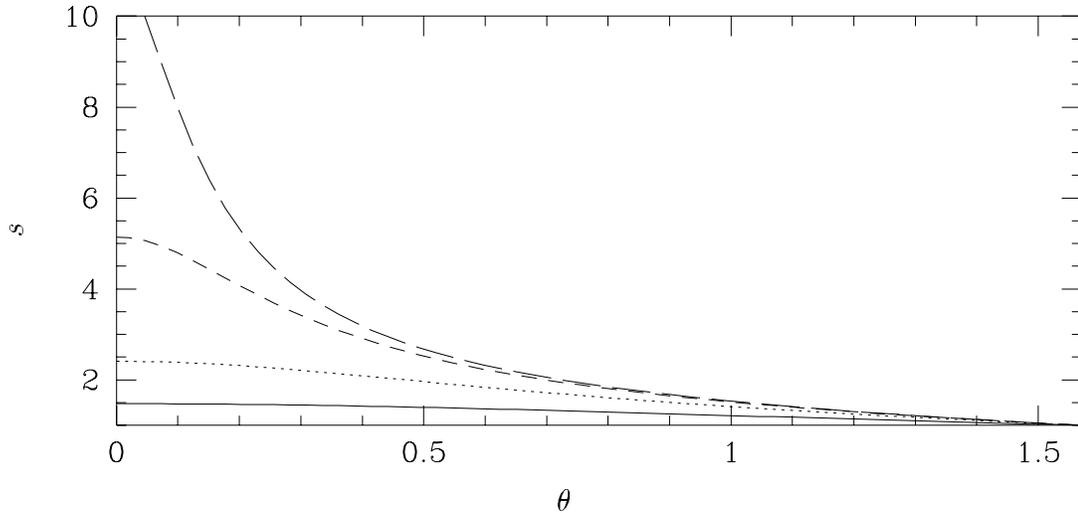
FIGURE 6. Maximum eigenvalue  $s$  of the amplification matrix  $\mathbf{g}$  for different orientations  $\theta$  of the Fourier mode  $\mathbf{k}$ . This case with no vorticity  $\Omega_0 = 0$ , at different crank angles: —,  $\omega t = \pi/4$ ; ·····,  $\omega t = \pi/2$ ; ----,  $\omega t = 3\pi/4$ ; - · - ·,  $\omega t = \pi$ .
