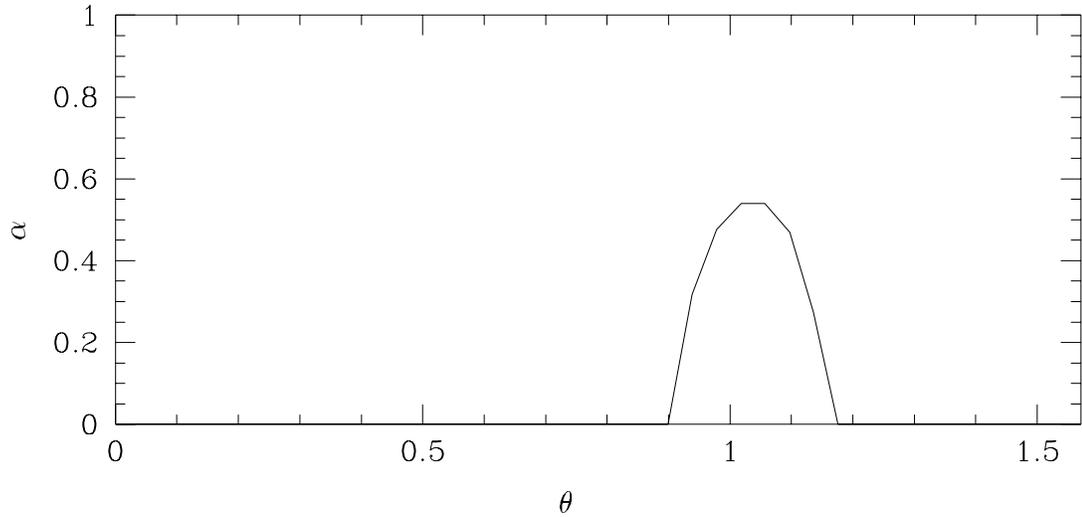
FIGURE 2. Elliptic vortex: Floquet parameter  $\alpha$  as a function of the orientation  $\theta$  of the Fourier mode  $\mathbf{k}$ . The peak value is located around  $\theta = \pi/3$  with a maximum close to  $9/16$  (see e.g. Waleffe, 1990).
