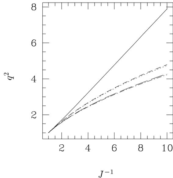
FIGURE 7. Evolution of the normalized kinetic energy for the compressed tumble vortex, as a function of the volumetric ratio  $J^{-1}$ , with  $J^{-1} = 10$  at the end of the compression. —,  $\Omega_0 = 0$ ; ·····,  $\Omega_0 = 10$ ; ----,  $\Omega_0 = 100$ ; - - - -,  $\Omega_0 = 500$ ; — · —,  $\Omega_0 = 1000$ .
