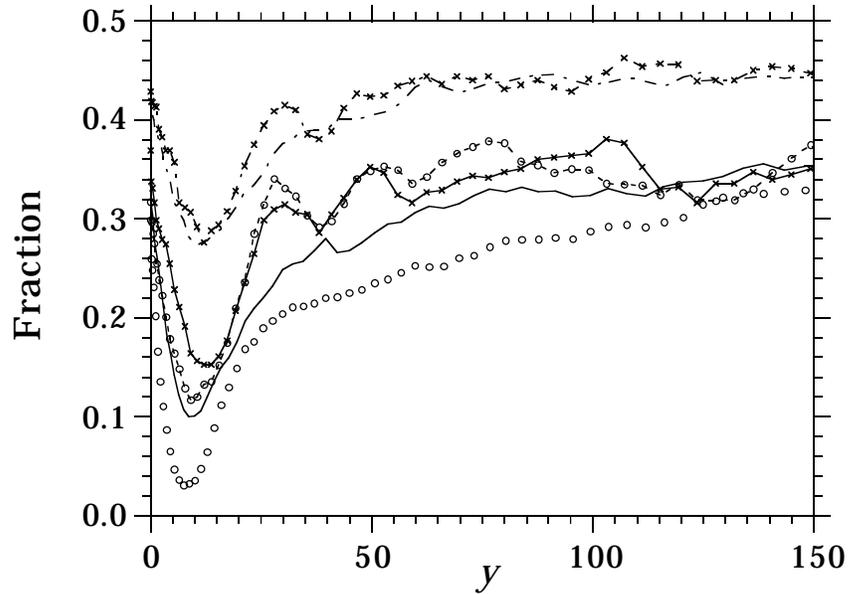
FIGURE 1.  $y$ -profiles of the fraction of grid points in each  $x - z$  plane where the SGS production term,  $P < 0$  from channel flow.  $\cdots \circ \cdots$ , Exact (low);  $-\times-$ , Bardina (low);  $--\times--$ , F-Bardina (low);  $\circ$ , Exact (high);  $----$ , Bardina (high);  $---$ , F-Bardina (high).
