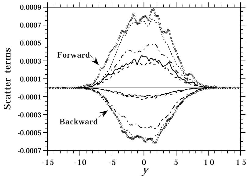
FIGURE 8. Decomposition of the plane-averaged  $P_{ij}$  terms obtained from the DNS exact data from high  $Re_\tau$  mixing layer. ---, (1,1); —, (1,2); o, (2,2); ----, (2,3); ..... , (3,3).
