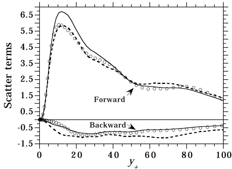
FIGURE 2. Decomposition of the plane-averaged SGS production term  $P$  obtained from the DNS exact data and obtained using different models from low  $Re_\tau$  channel flow. Symbols:  $\circ$ , Exact;  $----$ , Bardina;  $---$ , F-Bardina.
