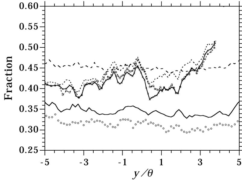
FIGURE 5.  $y$ -profiles of the fraction of grid points in each  $x - z$  plane where the SGS production term  $P < 0$  from mixing layer.  $\cdots \circ \cdots$ , Exact (low);  $\cdots \times \cdots$ , Bardina (low);  $-\times -$ , F-Bardina (low);  $\circ$ , Exact (high);  $-\times -$ , Bardina (high);  $---$ , F-Bardina (high).
